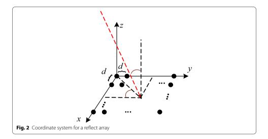
given that the element spacing d is equal over the x and y planes. When an EM wave impinges a planar array from the direction defined with the angle between the z-axis and the propagation direction of the wave ( $\varphi$ ) and the propagation direction in x-y plane ( $\varphi$ ), the signal components on the x-y plane are
