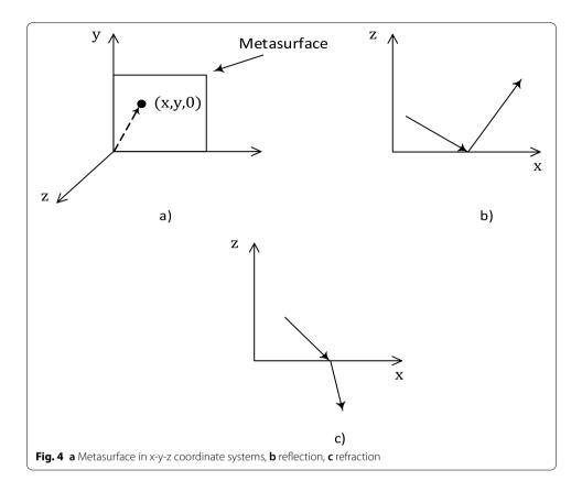
EM waves to any other directions. However, when an appropriately designed thin sheet is placed between the two materials, it is possible to control the behavior of the EM waves above and below the sheet more freely [25–29]. The engineered thin sheets with designed reflective, refractive and absorption properties are called metasurfaces.
