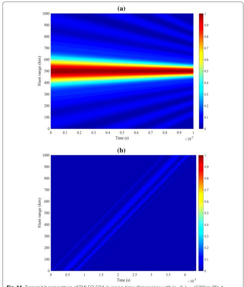
**Fig. 11** Transmit beampattern of TMLFO-FDA in range-time dimensions with  $(r_d, \theta_d) = (500 km, 0^\circ)$ . **a** Original time-invariant beampattern. **b** Corresponding correct beampattern
