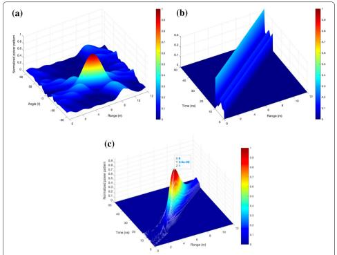
Fig. 12 Significance of the wave propagation effect. a C-TMOFO FDA original time-invariant beampattern. b C-TMOFO FDA corrected time-variant beampattern. c Original time-variant beampattern of the short-range FDA radar based on arc-tangent function
