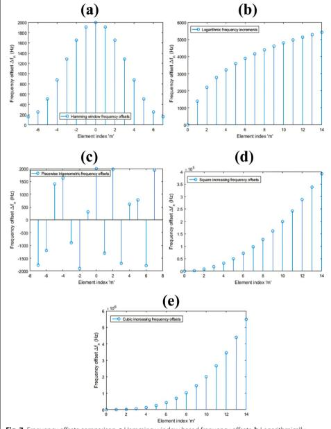
**Fig. 7** Frequency offsets comparison. **a** Hamming window based frequency offsets. **b** Logarithmically increasing frequency offsets. **c** Piecewise trigonometric frequency offsets. **d** Square increasing frequency offsets. **e** Cubic increasing frequency offsets
