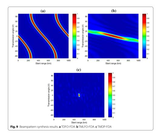
due to the high spatial peak sidelobe levels (P-SLL) and a broader spatial half-power beamwidth (HPBW). Furthermore, as Fig. 9c shows, the TMDP-FDA generate a well-shaped "dot" main beam and outperforms the other two schemes with a more focused beampattern due to multi-carrier architecture.
