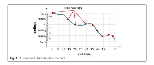
state. It is important to notice that the accuracy of  $R'_i$  can be regulated by the expert according the value assigned to  $\alpha$  which can be in  $[1, \mathcal{F}]$ ; 1 means that all readings are belonging to the same range  $[r_{min}, r_{max}]$  while  $\mathcal{F}$  indicates that all the collected data will send to the sink. Thus, more the value of  $\alpha$  is, more the accuracy of sent data is.
