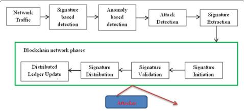
**Fig. 1** System architecture of proposed system BC-HyIDS using blockchain. The top view of the architecture which elaborates all the phases of prototype. Each step of the architecture is explained including blockchain framework. All the steps included in blockchain framework are explained in block. This framework will provide security to the system such that attackers will not able to penetrate attacks in network. This framework provides immutable data exchange
