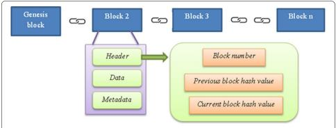
**Fig. 6** Block structure for hyperledger blockchain used in BC-HyIDS. Hyperledger blockchain along with block structure is shown. First block of this blockchain is genesis block. Each block consists of header, data and metadata. Each block is connected with other using hash functions. Unique identification is given to each block called block number
