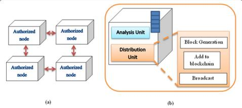
**Fig. 5** Blockchain framework: **a** blockchain network of BC-HyIDS and **b** individual node structure. BC-HyIDS system is a private blockchain network implemented using Hyperledger platform. As it is a private and permissioned network it consists of only authorized nodes. All nodes are connected to each other in a chain. Each node is able to do all functionality using analysis and distribution unit
