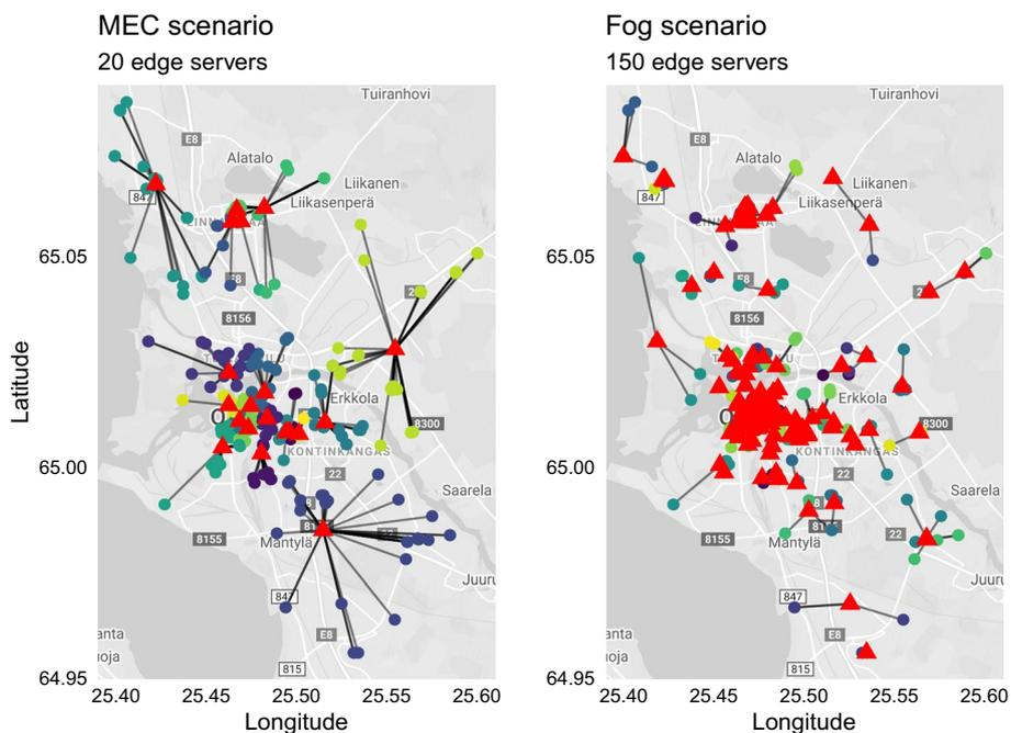
**Fig. 3** Location of edge servers and the allocation of APs to edge servers
