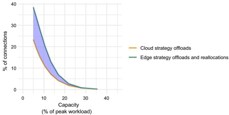
**Fig. 5** Superfluous reallocations. The difference (blue area) between the number of offloads for cloud strategy (orange line) and the number of reallocations and offloads for an edge strategy (green line) is the number of superfluous reallocations, shown here as a proportion of all connections. (Figure originally in [10].)
