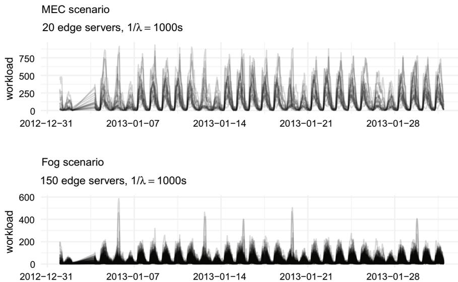
**Fig. 4** Workload on edge servers for MEC and Fog, with duration mean 1000s, during first weeks of the observation period 2013–2014. A service break is clearly visible in the first week
