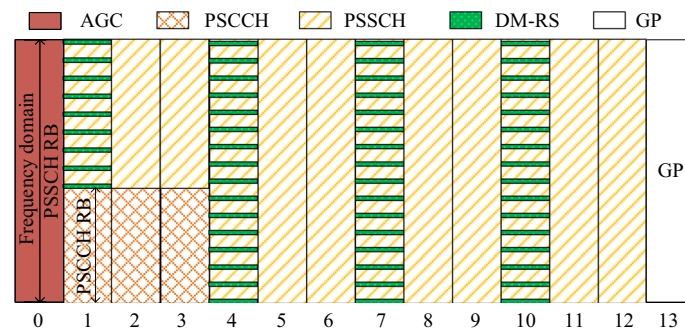
Fig. 2 Sketch map of the PSSCH time-frequency structure
