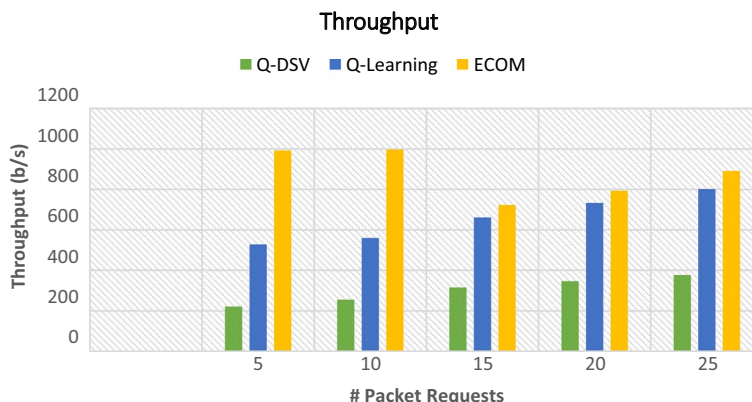
Fig. 7 Throughput in bps obtained by the ECOM proposed model. The result of the throughput for the proposed model compared to two other models
