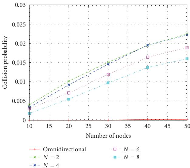
FIGURE 7: Collision probability as a function of the number of nodes in the case of omnidirectional and directive antennas with  $\pi$ ,  $\pi/2$ ,  $\pi/3$ , and  $\pi/4$  main lobes for  $T_f = 93$  seconds and  $\delta = 3\%$ .
