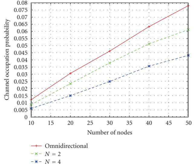
FIGURE 8: Channel occupation probability as a function of the number of nodes in the case of omnidirectional and directive antennas with  $\pi$  and  $\pi/2$  main lobes for  $T_f = 93$  seconds and  $\delta = 3\%$ .
