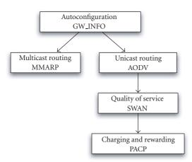
FIGURE 3: Functional architecture with protocols included.
