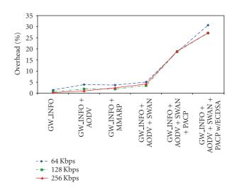
FIGURE 12: Cumulative overhead with the increase of functionalities.
