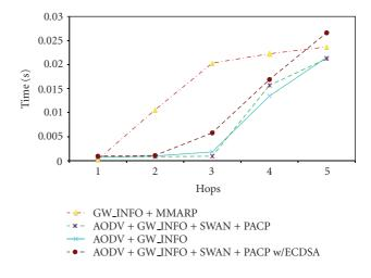
FIGURE 11: Cumulative jitter for the 256 kbits traffic profile.
