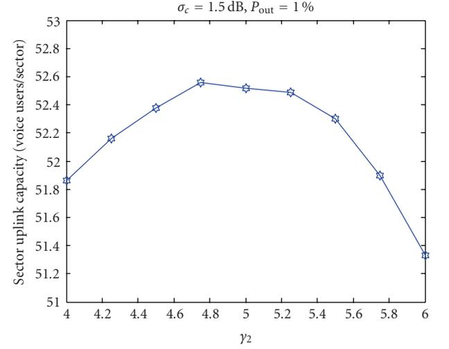
FIGURE 13: Effect of the propagation exponent  $\gamma_2$  on the sector uplink capacity.
