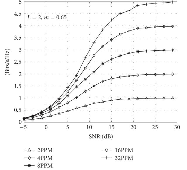
FIGURE 3: Capacity of a UWB system with PPM over a multipath fading channel with  $L = 2$  and  $m = 0.65$ .
