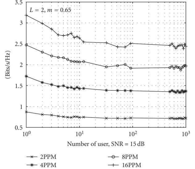
FIGURE 9: Relationship between channel capacity and number of users for a multiple access UWB system with PPM over a multipath fading channel,  $L = 2$ ,  $m = 0.65$ ,  $G = 100$ ,  $P_x = -11$  dBm, and SNR = 15 dB.
