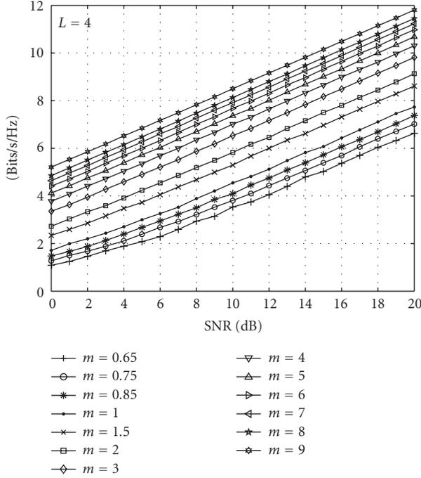
FIGURE 1: UWB multipath fading channel capacity with  $L = 4$ .
