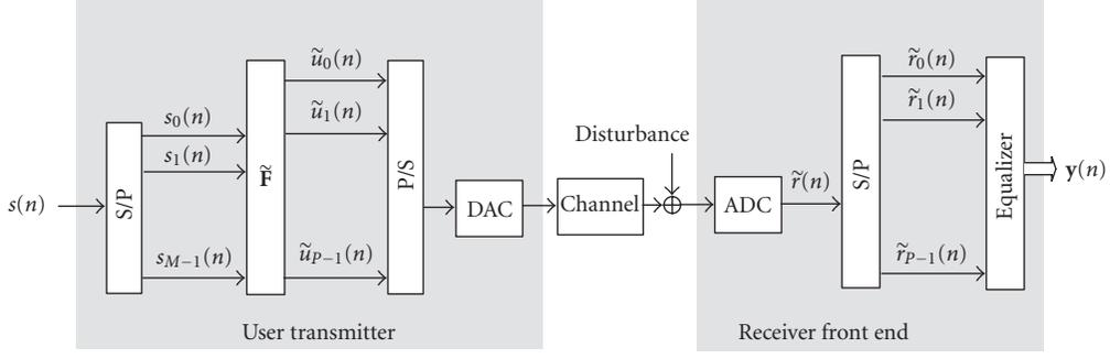
FIGURE 1: MC transceiver.
