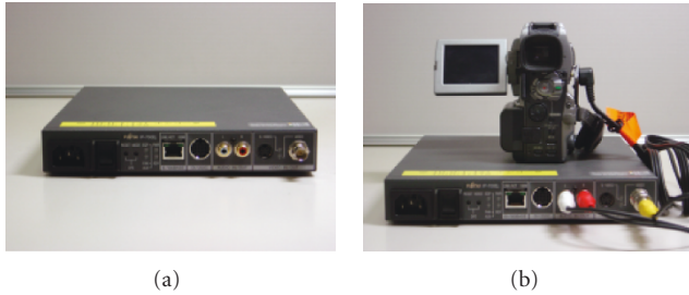
FIGURE 10: MPEG-2 encoder and decoder: (a) encoder, decoder unit, (b) camcorder with encoder.
