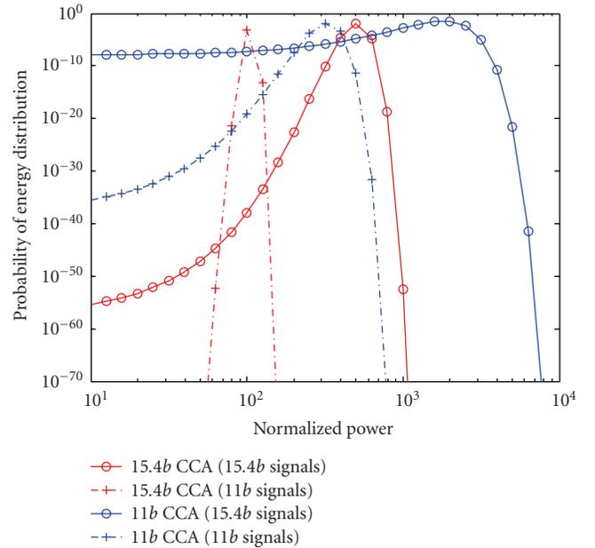
FIGURE 3: Collected power distributions of energy-based CCA over a free channel per different underlying signals.
