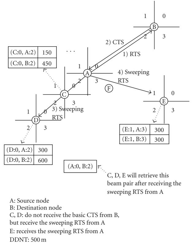
FIGURE 14: Illustration of the CA mechanism.
