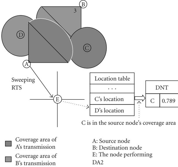
While A is transmitting to B, C is regarded deaf, but D is not regarded deaf; D is able to receive the RTS from E and beamform to E for reception, while B receives from A
