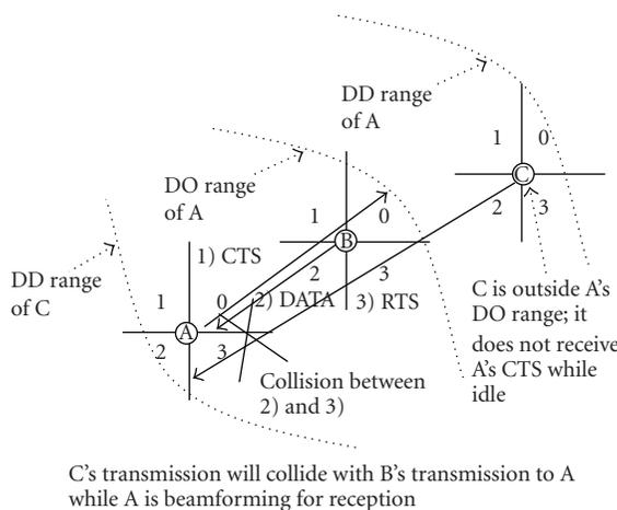
FIGURE 7: Illustration of first type of hidden terminal problems.
