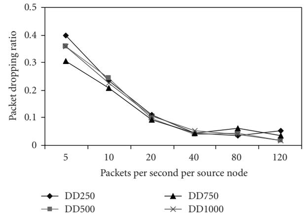
FIGURE 23: Effect of different DDNTs on the CA mechanism.
