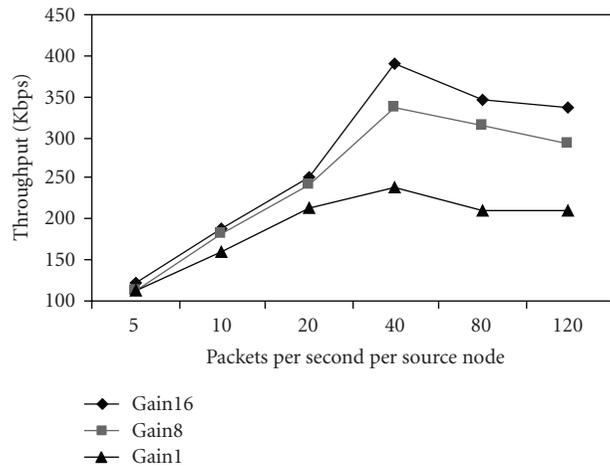
FIGURE 25: Throughput of DMAC-DACA with different antenna gains.
