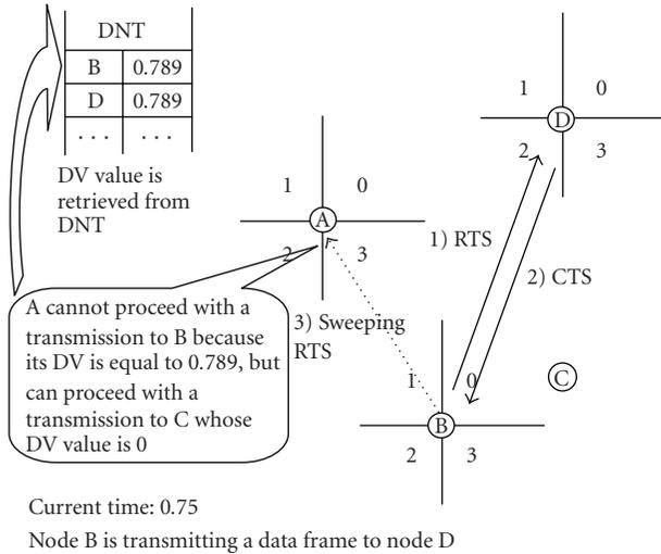
FIGURE 11: Illustration of the DA1 mechanism.
