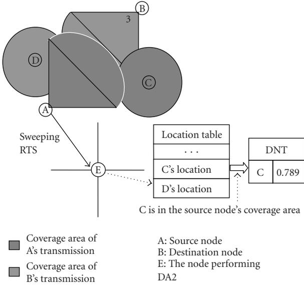
FIGURE 13: Illustration of the DA2 mechanism.
