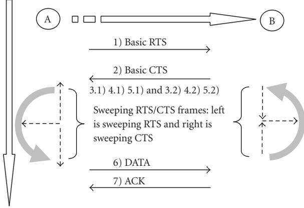
FIGURE 9: DMAC-DACA handshakes.
