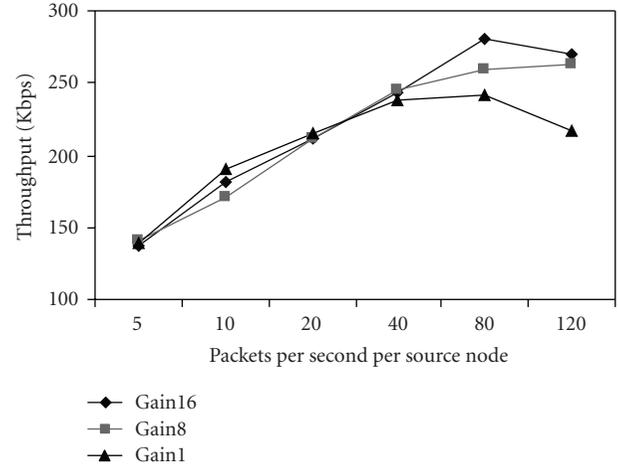
FIGURE 27: Throughput of OMNI IEEE 802.11 with different antenna gains.
