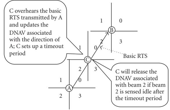
FIGURE 10: An example of DMAC-DACA reservation release.
