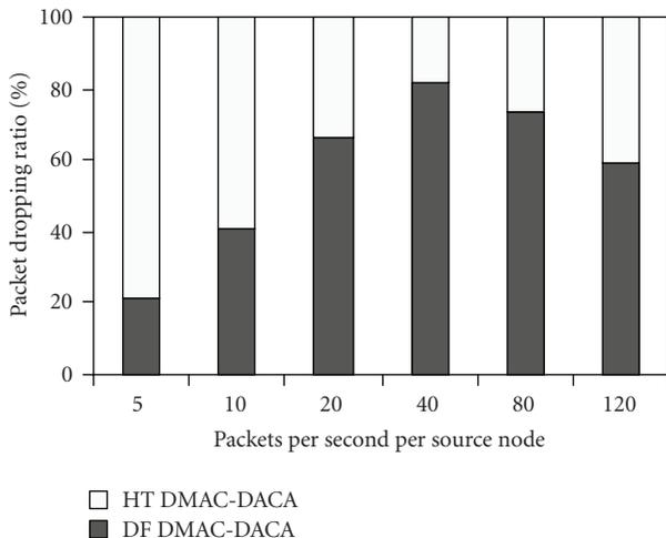
FIGURE 21: DMAC-DACA: deafness versus hidden terminals.
