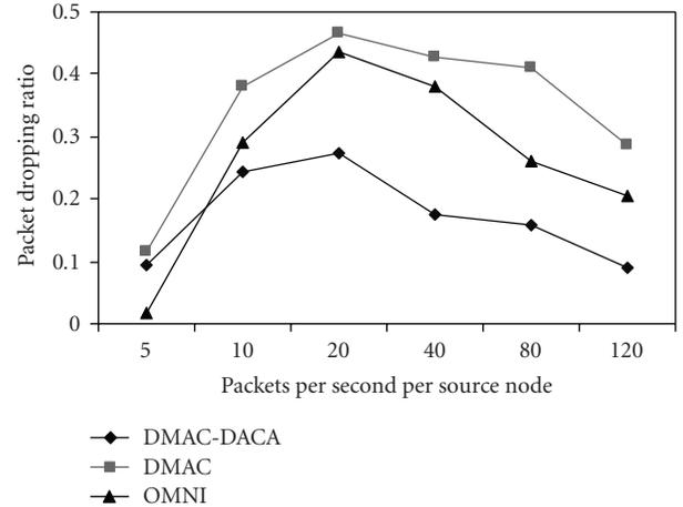
FIGURE 16: Effect of DMAC-DACA's DA mechanism.
