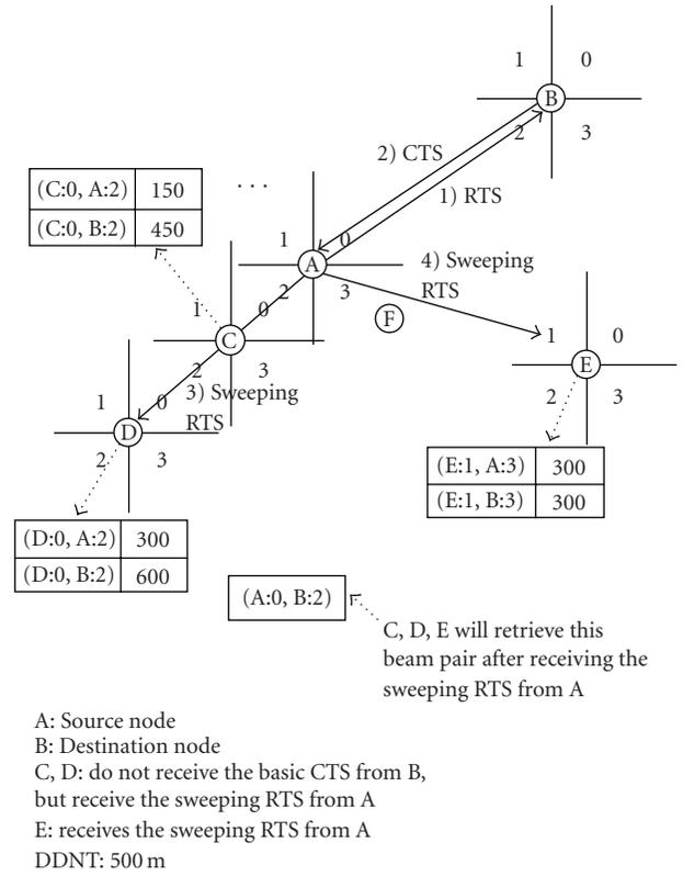
FIGURE 14: Illustration of the CA mechanism.
