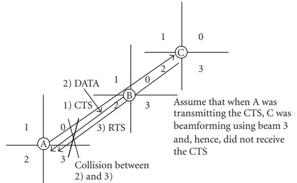
FIGURE 8: Illustration of second type of hidden terminal problem.
