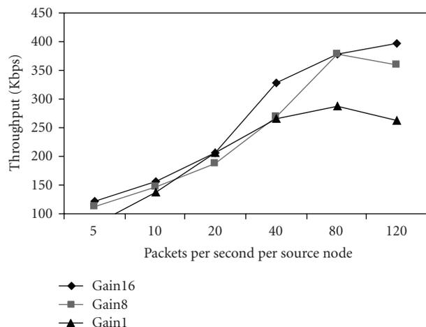
FIGURE 26: Throughput of DMAC with different antenna gains.
