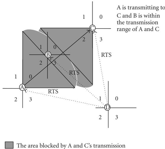
FIGURE 6: Illustration of the two types of deafness problems.
