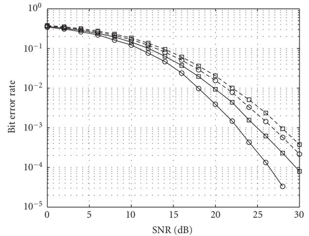
FIGURE 13: Performance of cluster-hopped RNS-FH OFDMA with different cluster sizes and different number of active users,  $f_D T_s = 0.01$ .
