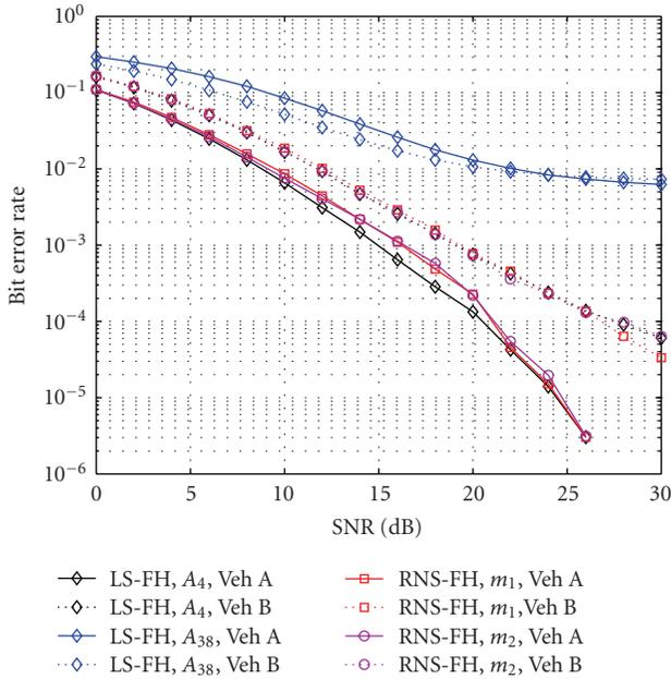
FIGURE 14: Performance of independent-hopped RNS-FH OFDMA versus LS-FH OFDMA,  $N = 110$ ,  $M = M_c = 10$ ,  $N_c = 11$ , LS  $A_4$  and  $A_{38}$  are used, different moduli sets  $m_1 = \{2, 55\}$  and  $m_2 = \{2, 11, 5\}$  are applied to construct RNS-FH patterns,  $f_D T_s = 0.01$ .
