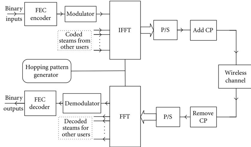
FIGURE 1: The block diagram of coded FH-OFDMA system.
