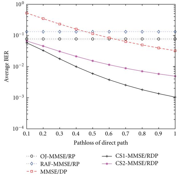
FIGURE 10: BER versus pathloss of direct path in uplink ( $\text{SNR}_1 = \text{SNR}_2 = 15$  dB).
