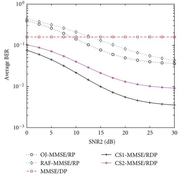
FIGURE 6: BER versus SNR of MS-RS link in uplink ( $p = 0.4$ ,  $\text{SNR}_1 = 15$  dB).
