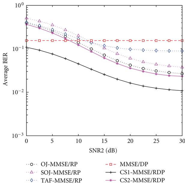
FIGURE 4: BER versus SNR of RS-MS link in downlink ( $p = 0.4$ ,  $\text{SNR}_1 = 15$  dB).
