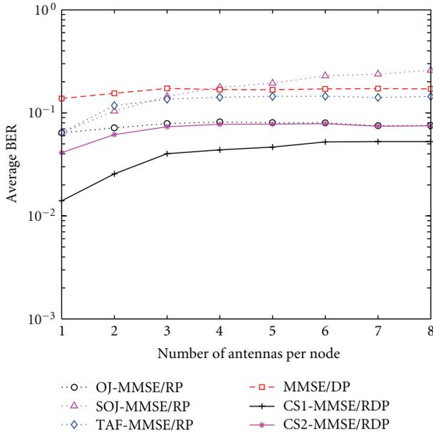
FIGURE 7: BER versus number of antennas in downlink ( $p = 0.4$ ,  $\text{SNR}_1 = \text{SNR}_2 = 15$  dB).
