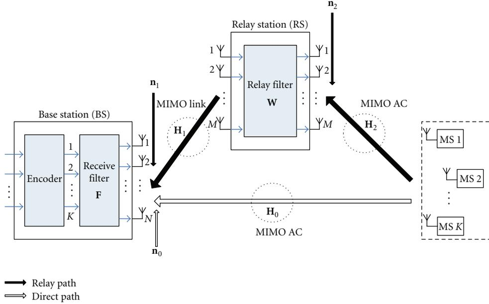
FIGURE 2: Multiuser cooperative MIMO relay system model in uplink.
