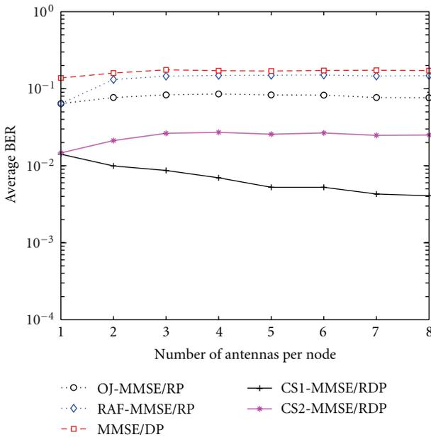
FIGURE 8: BER versus number of antennas in uplink ( $p = 0.4$ ,  $\text{SNR}_1 = \text{SNR}_2 = 15$  dB).
