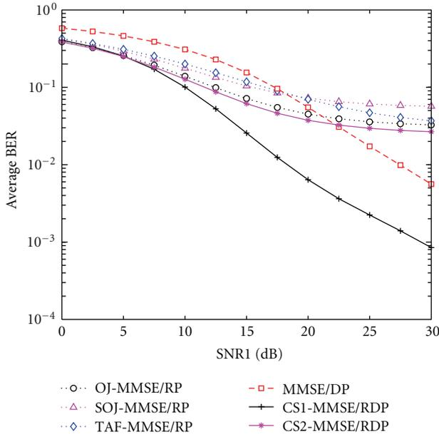
FIGURE 3: BER versus SNR of BS-RS link in downlink ( $p = 0.4$ ,  $\text{SNR}_2 = 15$  dB).
