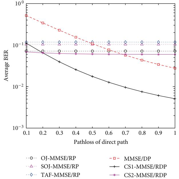
FIGURE 9: BER versus pathloss of direct path in downlink ( $\text{SNR}_1 = \text{SNR}_2 = 15$  dB).
