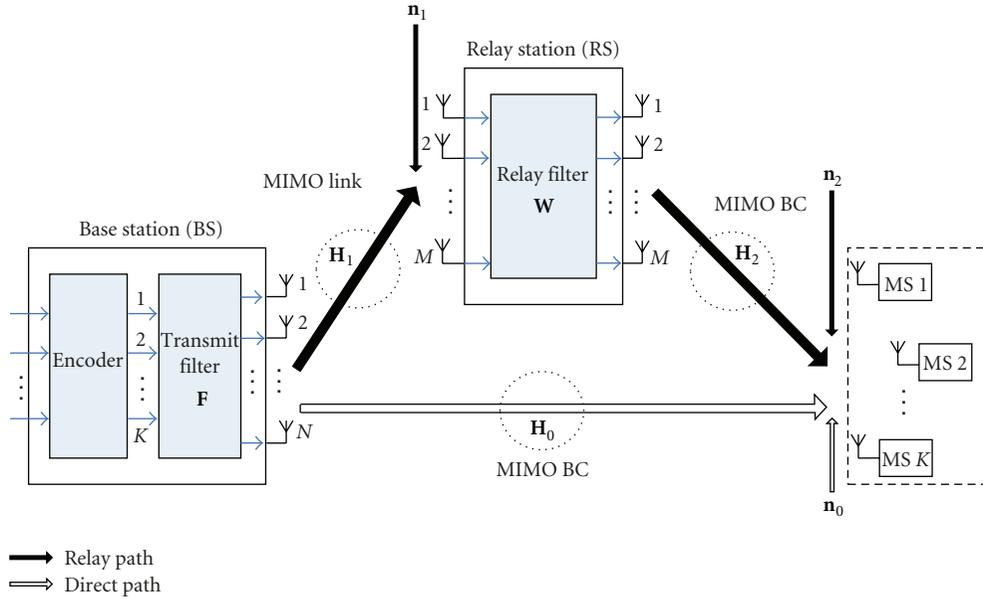
FIGURE 1: Multiuser cooperative MIMO relay system model in downlink.
