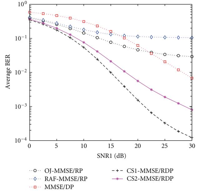
FIGURE 5: BER versus SNR of RS-BS link in uplink ( $p = 0.4$ ,  $\text{SNR}_2 = 15$  dB).
