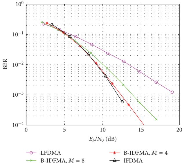
FIGURE 9: Coded SISO performance for B-IFDMA, IFDMA and LFDMA with nonperfect channel estimation, and  $Q = 32$  subcarriers assigned per user. The Block-LSE channel estimation performance results from Figure 8 are used. B-IFDMA uses block of sizes ( $M = 4, N_t = 6$ ) or ( $M = 8, N_t = 6$ ).
