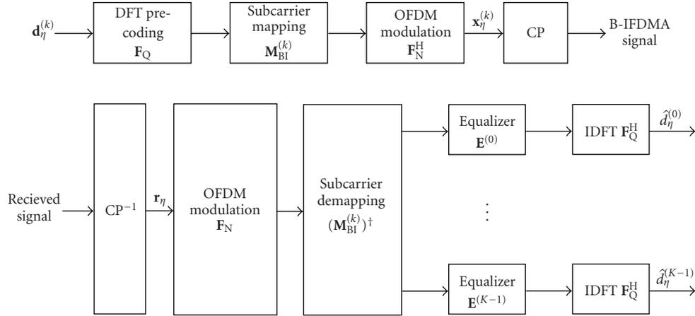
FIGURE 2: B-IFDMA transceiver, transmitter (top) and receiver (bottom). In case the same amount of resources are allocated per user, for each user  $k$  out of  $K$  uplink user terminals,  $Q$  out of  $N$  subcarriers are allocated by the subcarrier mapping matrix  $\mathbf{M}_{\text{BI}}^{(k)}$ . The allocated subcarriers consist of  $L$  blocks, each containing  $M$  adjacent subcarriers.
