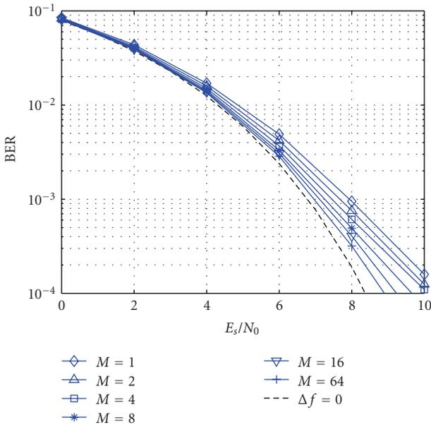
FIGURE 14: Performance for Doppler Spread with  $\Delta \bar{f}_{\text{CFO}}^{(k)} = 15\%$  relative carrier frequency offset per path for different numbers  $M$  of subcarriers per block, assuming  $N = 1024$  subcarriers and  $Q = 64$  subcarriers per user.
