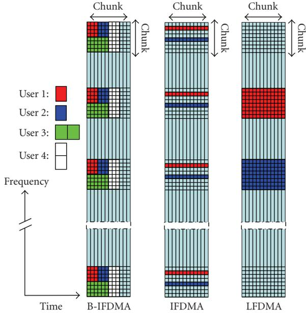
FIGURE 1: Illustration of B-IFDMA using  $M = 4$  subcarriers and  $N_t = 3$  OFDM symbols per subcarrier block within a time-frequency resource denoted as chunk. SC-FDMA with localized mapping (LFDMA) and SC-FDMA with distributed mapping (IFDMA) are shown for comparison. In B-IFDMA, high rate users are allocated more blocks within the chunks in either the time or the frequency direction. (A similar illustration is included in [12].)
