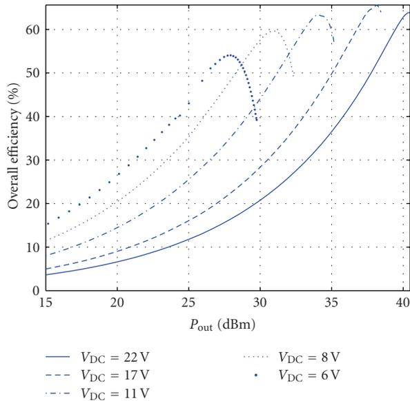
FIGURE 12: Illustration of overall efficiency as a function of output power for different amplifier drive voltages  $V_{DC}$  using the HPA in [42], where  $V_{DC} = 22$  V is the highest possible drive voltage.
