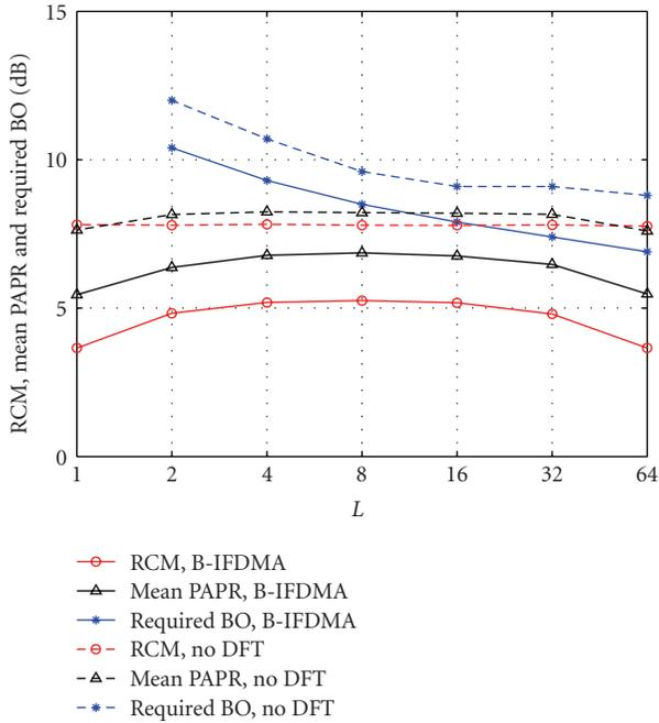
FIGURE 11: Results for the analysis of the envelope fluctuations of B-IFDMA transmit signals with  $Q = 64$  (with DFT) compared to signals without DFT precoding for different numbers  $L$  of subcarriers per block using different metrics.
