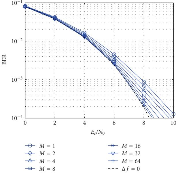
FIGURE 13: Performance for  $\Delta \bar{f}_{\text{CFO}}^{(k)} = 10\%$  maximum relative CFO for different numbers  $M$  of subcarriers per block, assuming  $N = 1024$  subcarriers and  $Q = 64$  subcarriers per user.
