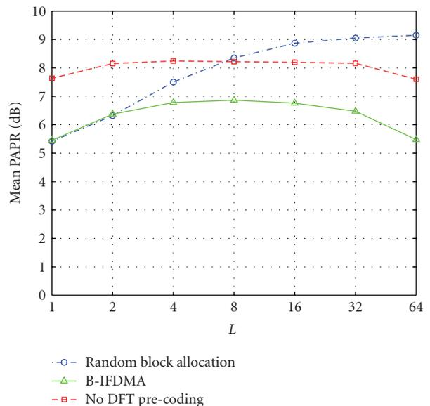
FIGURE 10: Mean PAPR of B-IFDMA transmit signals with  $Q = 64$  as a function of number of blocks  $L$  compared to the corresponding schemes without DFT precoding and schemes with random allocation of the subcarrier blocks.
