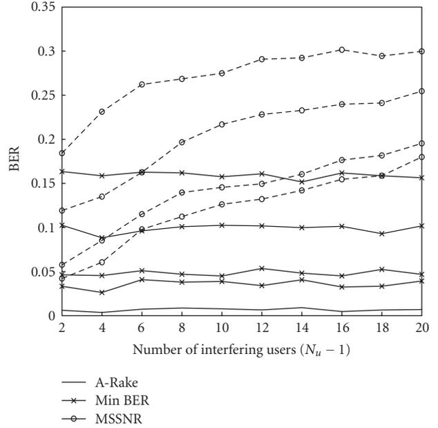
FIGURE 5: The BER performance of different Rake receivers and TEQ designs at SNR = 15 dB and  $N = 32$  versus the increasing number of users.
