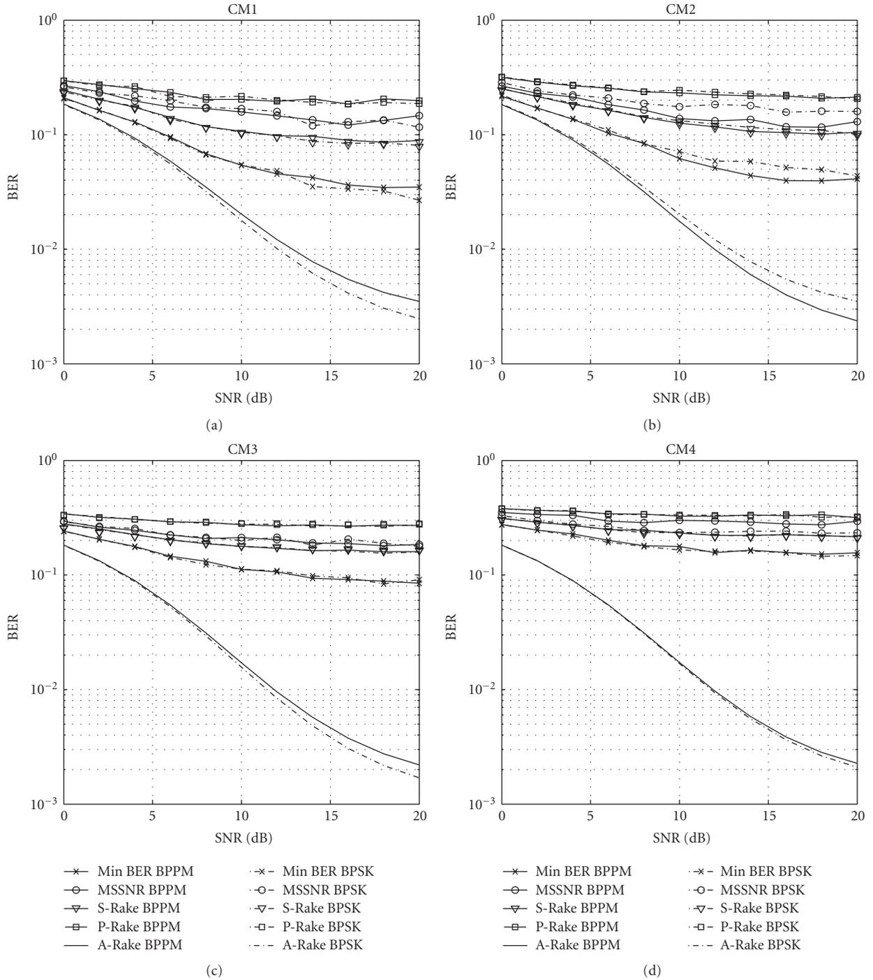
FIGURE 3: The BER performance of different Rake receivers and TEQ designs with a fixed number of interfering users and TEQ length.
