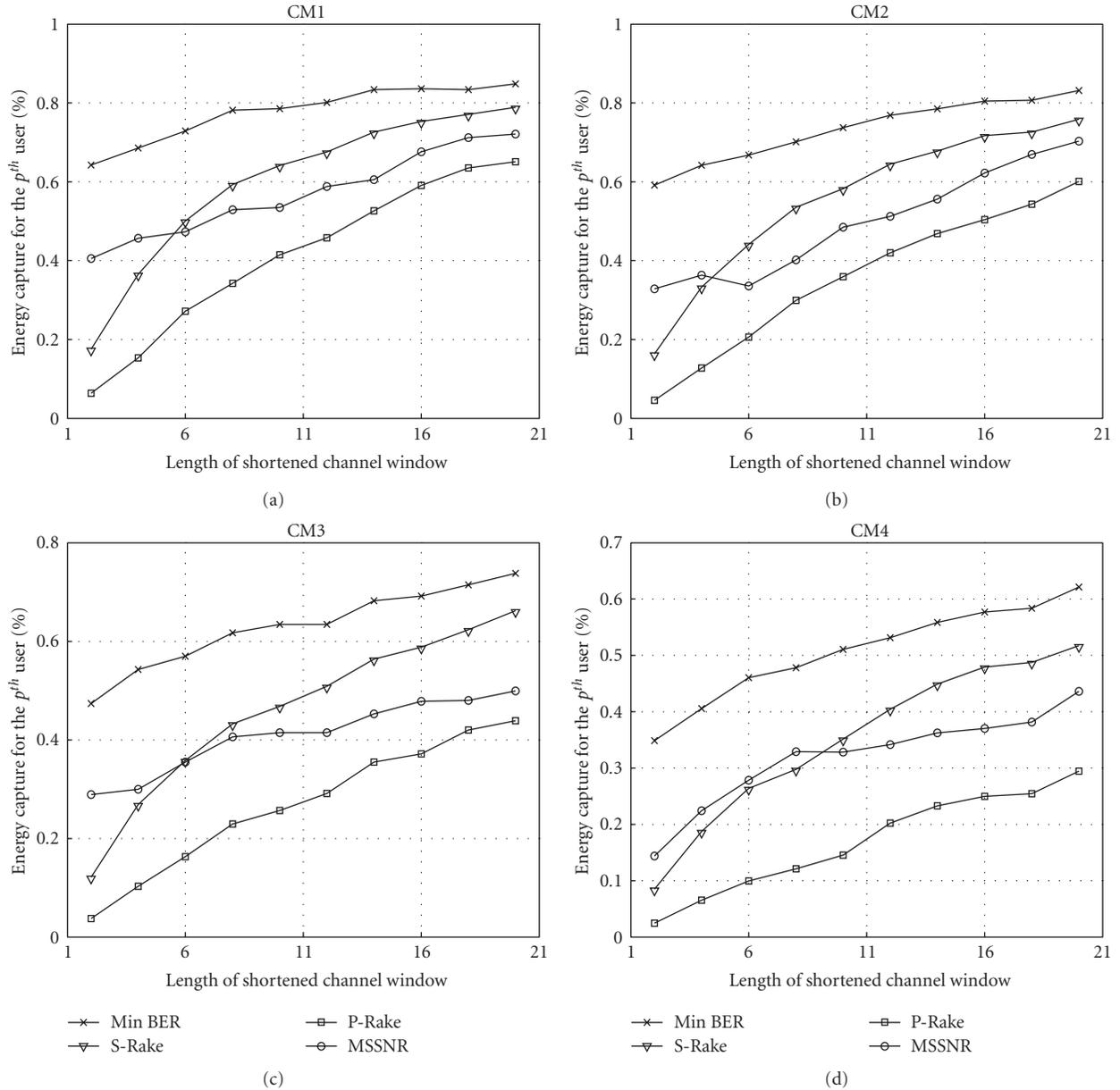
FIGURE 6: The energy capture performance of different Rake receivers and TEQ designs at SNR = 15 dB,  $N = 32$ , and  $N_u = 10$  versus the length of shortened channel window  $\ell$ .
