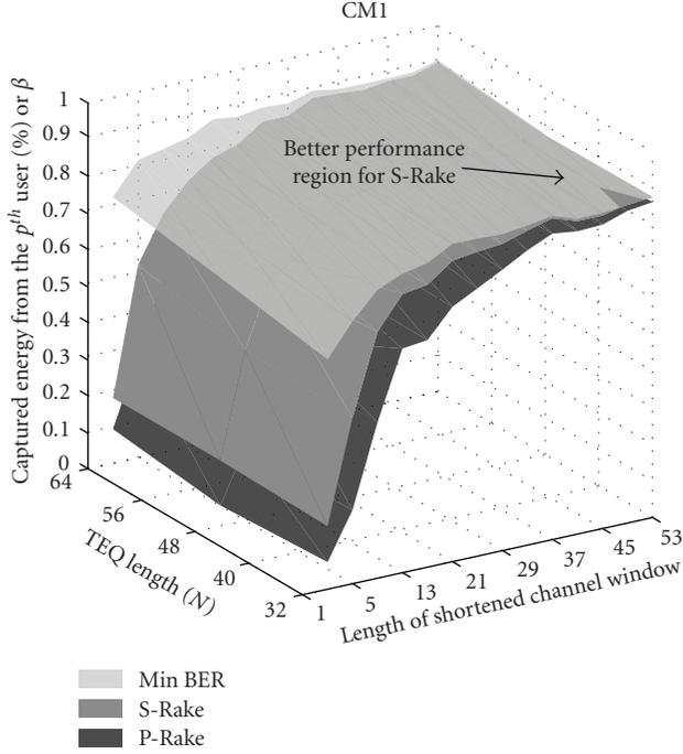
FIGURE 1: The energy capture performance of different Rake receivers and the proposed TEQ at SNR = 15 dB and  $N_u = 10$  versus the length of shortened channel window  $\ell$  and the TEQ length  $(N)$ .
