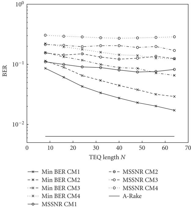
FIGURE 4: The BER performance of different Rake receivers and TEQ designs at SNR = 15 dB with a fixed number of interfering users versus increasing TEQ length.
