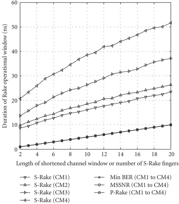
FIGURE 2: The duration of operational window for different Rake structures and TEQ designs.
