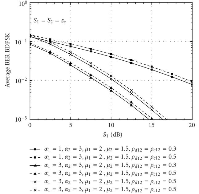
FIGURE 3: Average bit error probability (ABER) versus average SIRs at the input branches of the balanced dual-branch switched-and-stay combiner,  $S_1$ , for BDPSK modulation scheme and several values of  $\rho_{d12}$ ,  $\rho_{c12}$ ,  $\mu_1$ ,  $\mu_2$ ,  $\alpha_1$ , and  $\alpha_2$ .
