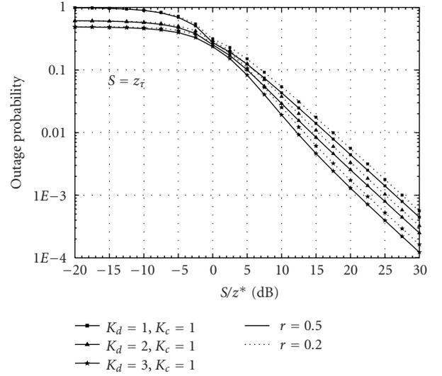
FIGURE 1: Outage probability ( $P_{out}$ ) versus normalized outage threshold for the balanced dual-branch SSC diversity receiver and different values of parameters  $r$  and  $K_d$ .
