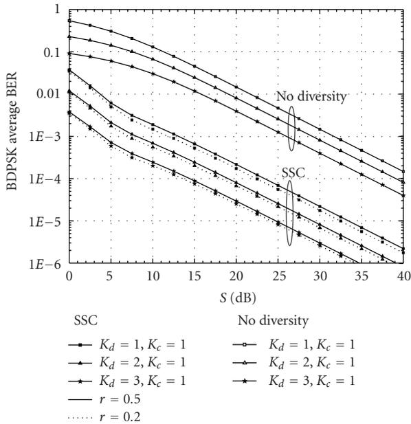
FIGURE 3: Average bit error probability (ABER) versus average SIRs at the input branches of the balanced dual-branch switched-and-stay combiner,  $S$ , for BDPSK modulation scheme and several values of parameters  $r$  and  $K_d$ .
