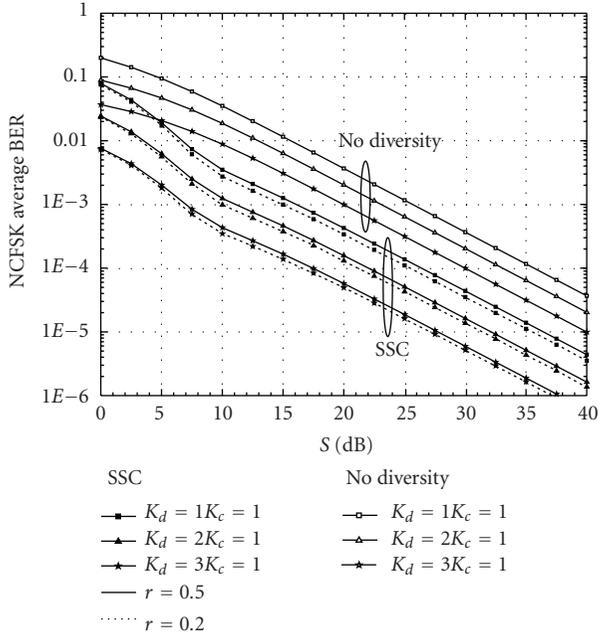
FIGURE 2: Average bit error probability (ABER) versus average SIRs at the input branches of the balanced dual-branch switched-and-stay combiner,  $S$ , for NCFSK modulation scheme and several values of parameters  $r$  and  $K_d$ .
