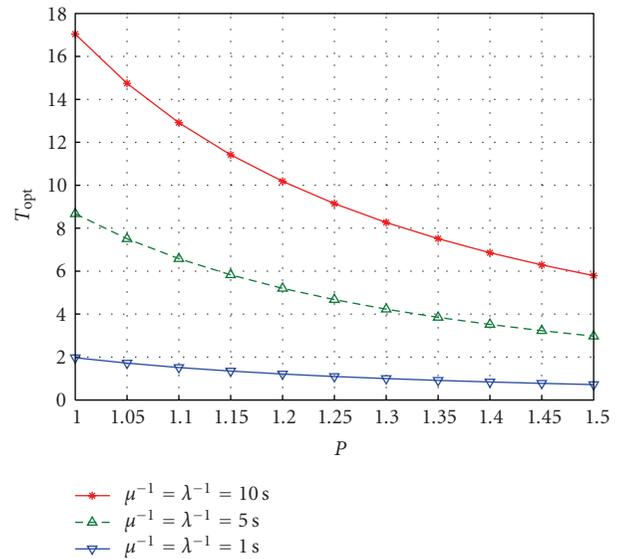
FIGURE 5: The optimal  $T_{\text{opt}}$  versus  $P$  for different holding times.
