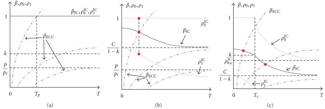
FIGURE 3: Illustration of the relationship of IC and ECC under access policy  $\pi_2$ .  $\beta_{\text{ECC}}$  is the maximal  $\beta$  under ECC.  $\beta_{\text{IC}}$  is the maximal  $\beta$  under IC and  $\rho_0^{\text{IC}}, \rho_1^{\text{IC}}$  are its corresponding transmission allocation.
