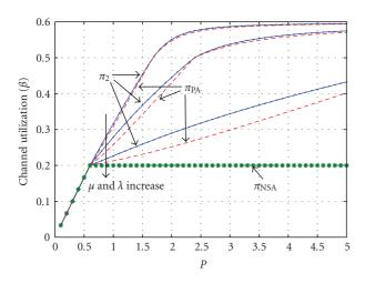
FIGURE 16: The channel utilization  $\beta$  under access policy  $\pi_2$ ,  $\pi_{PA}$  and  $\pi_{NSA}$ .
