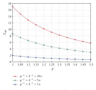
FIGURE 5: The optimal  $T_{opt}$  versus P for different holding times.
