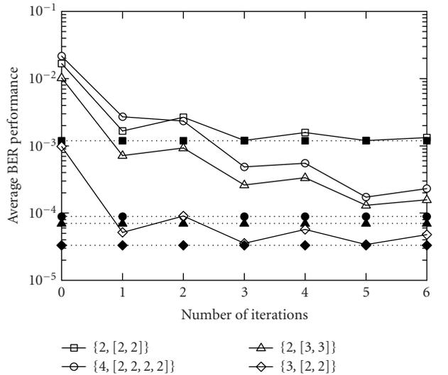
FIGURE 7: Average BER performance of the proposed iterative Pinv-MRC method for various number of iterations at SNR = 8 dB and 4-QAM.
