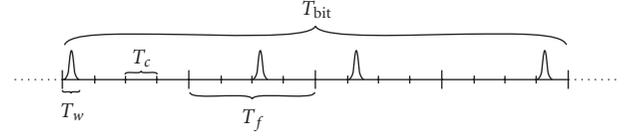
FIGURE 1: Representation of a transmitted bit. In the above example,  $b = 1$  and  $c_\ell(m) = \{0, 2, 1, 3\}$ .
