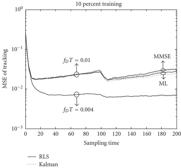
FIGURE 6: MSE of the proposed algorithm and Kalman filter for  $2 \times 4$  MIMO channel while 10% data is training.
