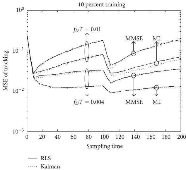
FIGURE 7: MSE of the proposed algorithm and Kalman filter for  $4 \times 4$  MIMO channel while 10% data is training.
