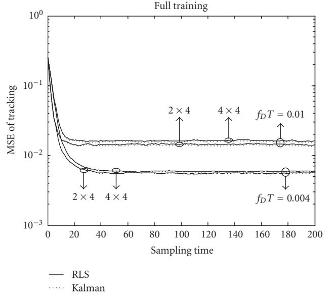
FIGURE 5: MSE of the proposed algorithm and Kalman filter while 100% data is training.
