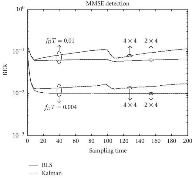
FIGURE 3: BER of the proposed algorithm with MMSE detection.
