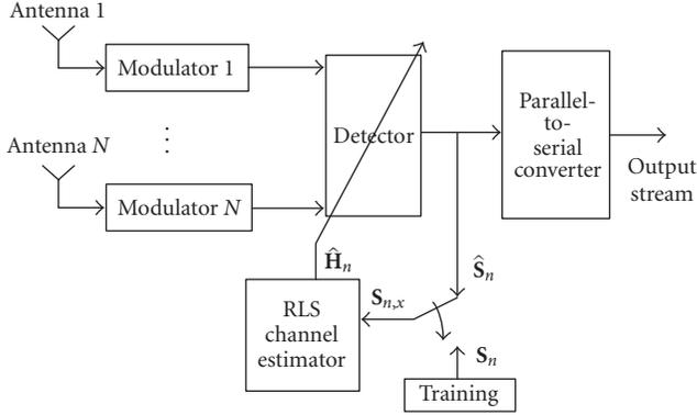
FIGURE 2: Block diagram of the receiver.
