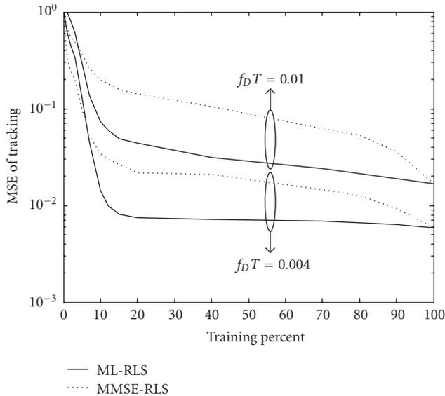
FIGURE 11: MSE of the proposed algorithm versus the training percent for  $4 \times 4$  MIMO channel.
