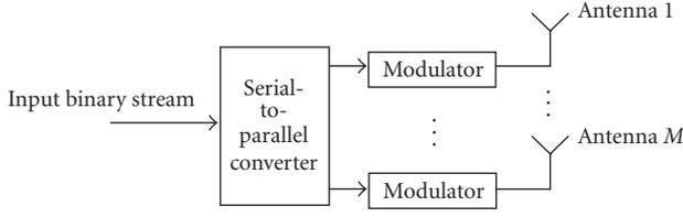
FIGURE 1: Block diagram of a simple spatial multiplexed MIMO transmitter.
