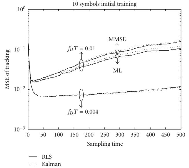
FIGURE 8: MSE of the proposed algorithm and Kalman filter for  $2 \times 4$  MIMO channel while the 10 first symbols are used as training.
