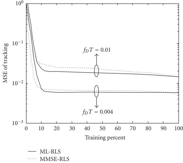
FIGURE 10: MSE of the proposed algorithm versus the training percent for  $2 \times 4$  MIMO channel.
