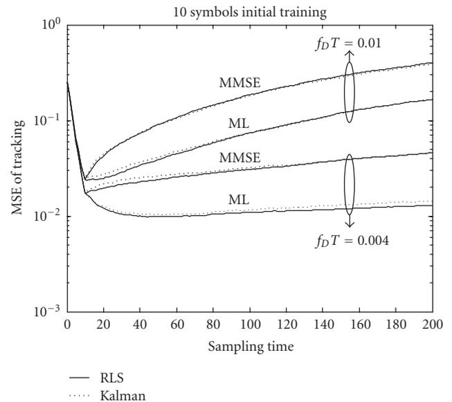
FIGURE 9: MSE of the proposed algorithm and Kalman filter for  $4 \times 4$  MIMO channel while the 10 first symbols are used as training.
