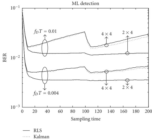
FIGURE 4: BER of the proposed algorithm with ML detection.
