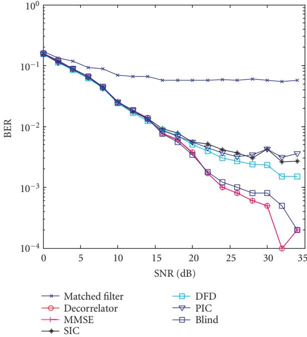
FIGURE 6: BER performance comparison between the proposed blind ICA multiuser receiver and the other receivers in a fast Rayleigh fading channel with the  $f_D = 1$  kHz,  $T_s = 10^{-2}$ , number of the users,  $K = 10$ , processing gain,  $N_{PG} = 31$ .
