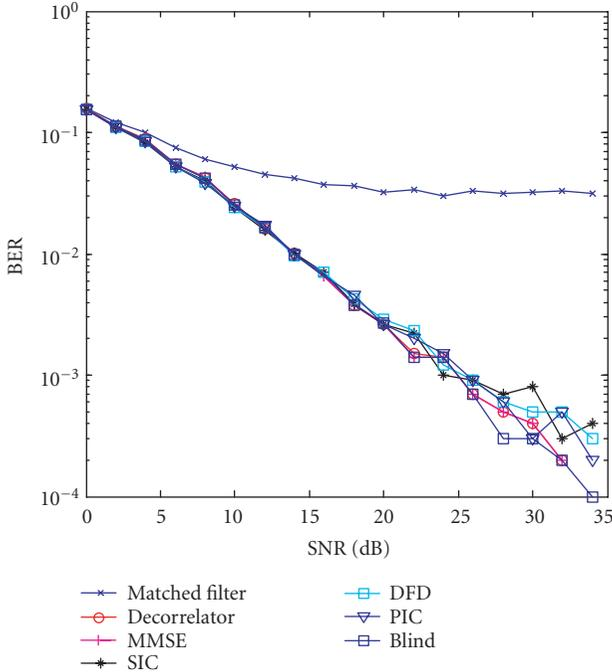
FIGURE 7: BER performance comparison between the proposed blind ICA multiuser receiver and the other receivers in a fast Rayleigh fading channel with the  $f_D = 100$  Hz,  $T_s = 10^{-2}$ , number of the users,  $K = 10$ , processing gain,  $N_{PG} = 127$ .
