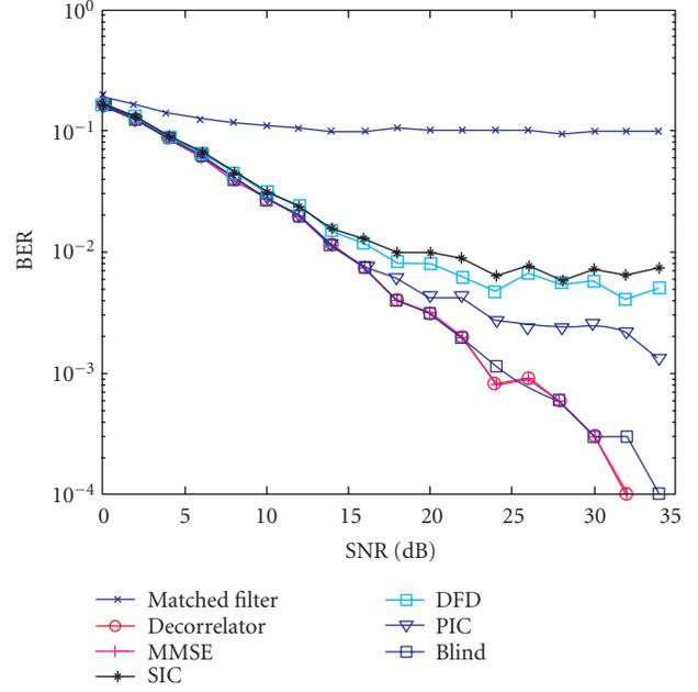
FIGURE 5: BER performance comparison between the proposed blind ICA multiuser receiver and the other receivers in a fast Rayleigh fading channel with the  $f_D = 1$  kHz,  $T_s = 10^{-2}$ , number of the users,  $K = 10$ , processing gain,  $N_{PG} = 127$ .
