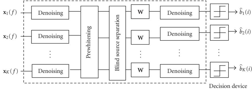
FIGURE 2: The proposed blind receiver consisting of PCA, ICA, and denoising stages.
