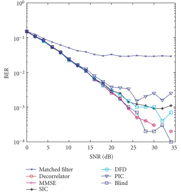
FIGURE 8: BER performance comparison between the proposed blind ICA multiuser receiver and the other receivers in a fast Rayleigh fading channel with the  $f_D = 100$  Hz,  $T_s = 10^{-2}$ , number of the users,  $K = 10$ , processing gain,  $N_{PG} = 31$ .
