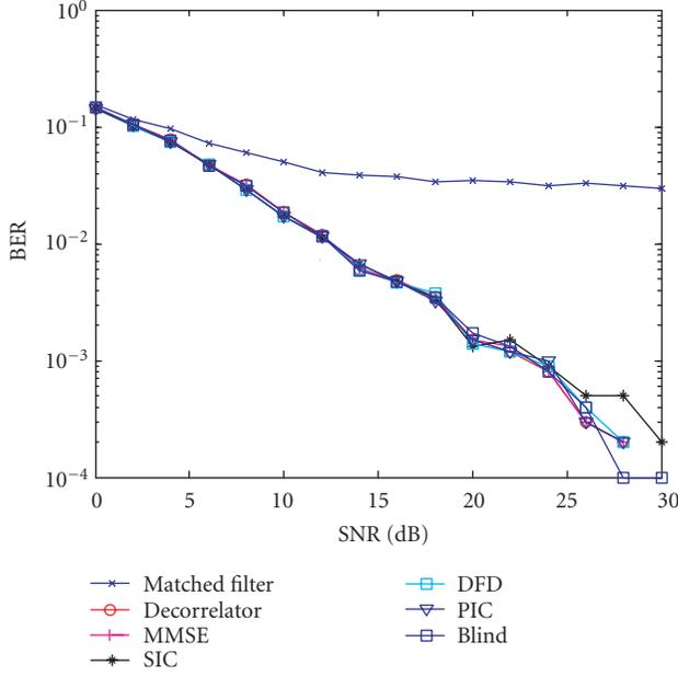
FIGURE 3: BER performance comparison between the proposed blind ICA multiuser receivers and the other conventional receivers in a slow-fading channel with the  $f_D = 10$  Hz,  $T_s = 10^{-4}$ , number of the users,  $K = 10$ , processing gain,  $N_{PG} = 127$ .
