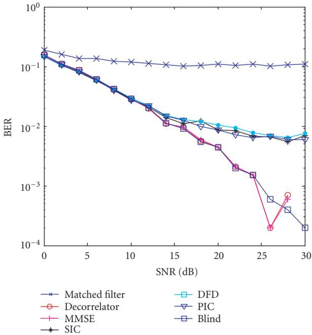
FIGURE 4: BER performance comparison between the proposed blind ICA multiuser receiver and the other receivers in a slow Rayleigh channel with the number of the users,  $K = 10$ ,  $f_D = 10$  Hz,  $T_s = 10^{-4}$ , processing gain,  $N_{PG} = 31$ .
