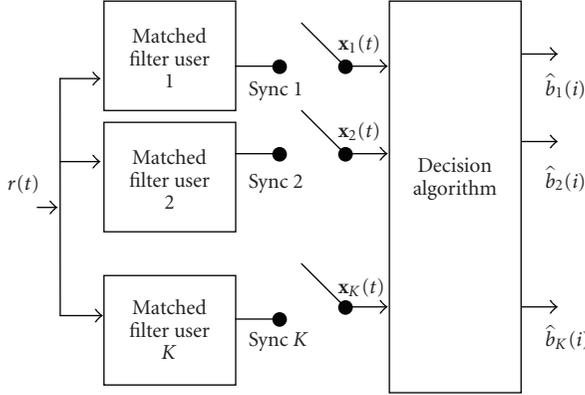
FIGURE 1:  $K$ -user detectors for multiple-access Gaussian channel.
