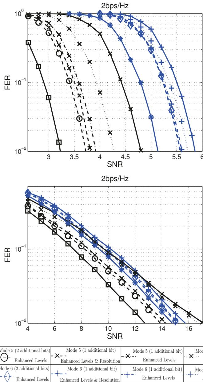
**Figure 9 Proposed precoder codebook.** Downlink channel with dual-antenna eNodeB and two single-antenna UEs. *Top figure* shows the results for fast fading channels while *bottom figure* illustrates the performance for slow fading channels. 3GPP LTE rate 1/3 turbo code is used with different puncturing patterns.
