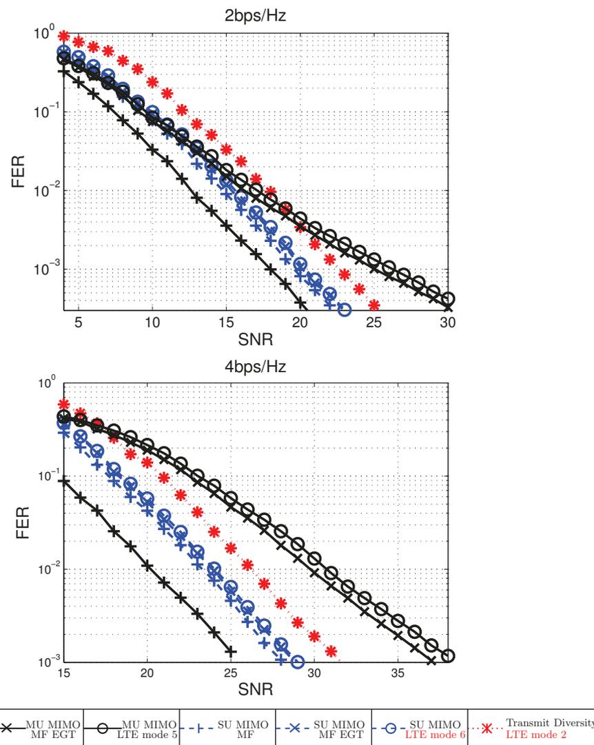
**Figure 7 Diversity in the single-user and multi-user MIMO modes.** Downlink slow fading channel (one channel realization per codeword) with dual-antenna eNodeB and two single-antenna UEs. 3GPP LTE rate 1/3 turbo code is used with different puncturing patterns.
