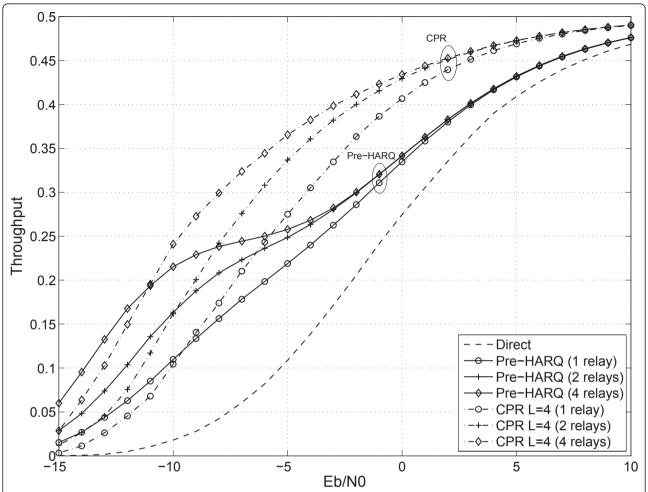
**Figure 4 Throughput performance of the direct transmission, Pre-HARQ, and CPR with** L = 4**.** The cooperative schemes are presented with 1, 2, and 4 relays, assuming that all relays are approximately at the same distance  $\delta = 0.5$  from the source.
