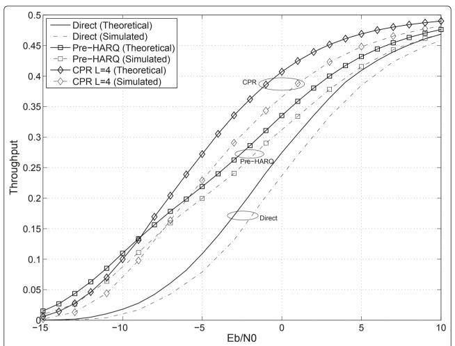
**Figure 7** Simulation results obtained using LDPC codes for the direct transmission, Pre-HARQ, and the proposed CPR scheme. The results are compared to the theoretical throughput derived from the outage analysis for each scheme.
