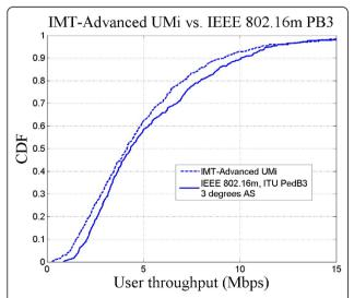
Figure 3 User throughput CDFs for the UMi test environment of IMT-Advanced and the IEEE 802.16 m PB3 and 3 degrees AS.
