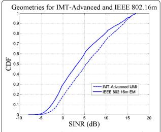
Figure 2 Geometries for the UMi test environment of IMT-Advanced and the IEEE 802.16 m evaluation methodology.
