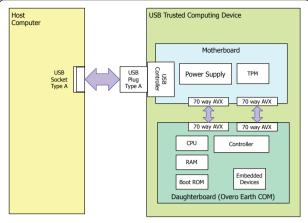
Figure 5 An implementation architecture of USB trusted platform computing device.
