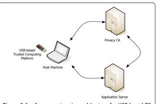
Figure 8 A reference enterprise architecture for USB-based TC platform.
