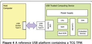
Figure 4 A reference USB platform containing a TCG TPM.
