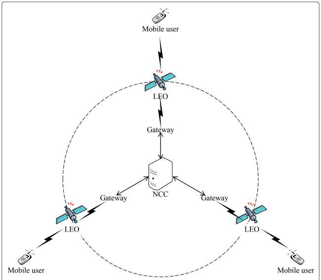
Figure 1 Overview of a simple mobile satellite communication network: wired secure network (solid lined) and wireless network (thunderbolt lined).
