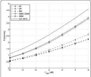
Figure 4 Average network spectral efficiency in terms of  $\Gamma_{\text{REF}}$  for the network model described in Figure 5.
