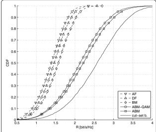
Figure 6 CDF of the network spectral efficiency with  $\Gamma_{\rm REF}=2$  dB, relay 1 located at (0,  $d_{\rm MAX}/3$ ), relay 2 at (0, 0), and relay 3 at (0,  $-d_{\rm MAX}$ ).
