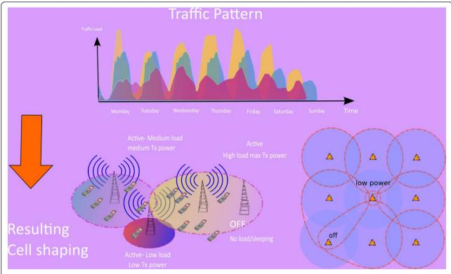
**Figure 5 Cell shape adaptation in function of traffic distribution**. The traffic pattern is the main input, which permits to shape the cell deployment, i.e. switching off the BSs or changing transmission power levels.
