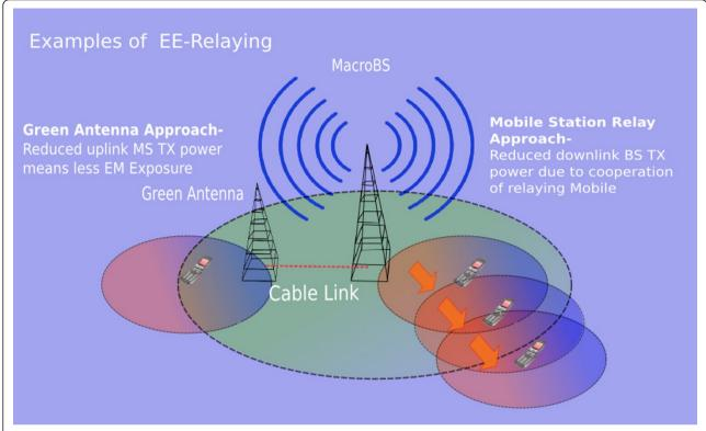
Figure 7 Two examples of relaying in the same figure: (left) a green antenna relay [38]; (right) downlink relaying using MSs as relays nodes [39].
