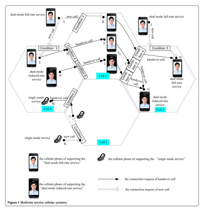
full-rate service" in point F of cell 1 changes into the "dual mode reduced-rate service" in point G of cell 2, and the handover connection request from point F to G in cell 2 is permitted. The location of the service type change is point C.
