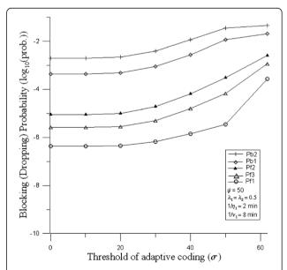
Figure 2 Blocking or dropping probability of cell 1 versus the adaptive coding threshold.
