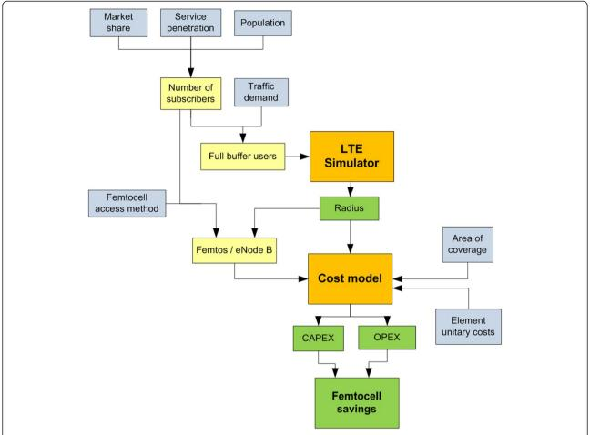
**Figure 2 Flow diagram used in the techno-economic model.** Assumptions and input values are shown in blue, intermediate calculations in orange, and final results in green.
