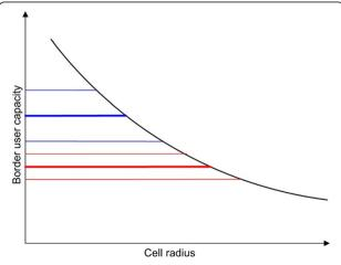
Figure 1 Cell-edge user throughput continuously decrease as a function of the cell radius.
