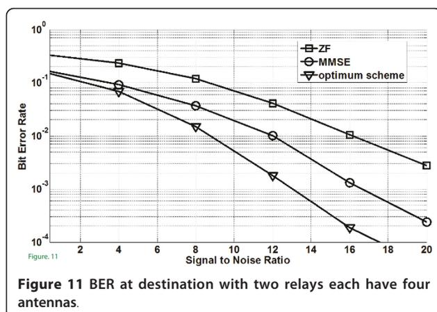
**Figure 11** BER at destination with two relays each have four antennas.
