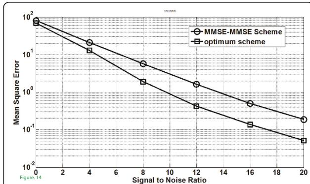
**Figure 14** MSE at destination with four relays each having four antennas.
