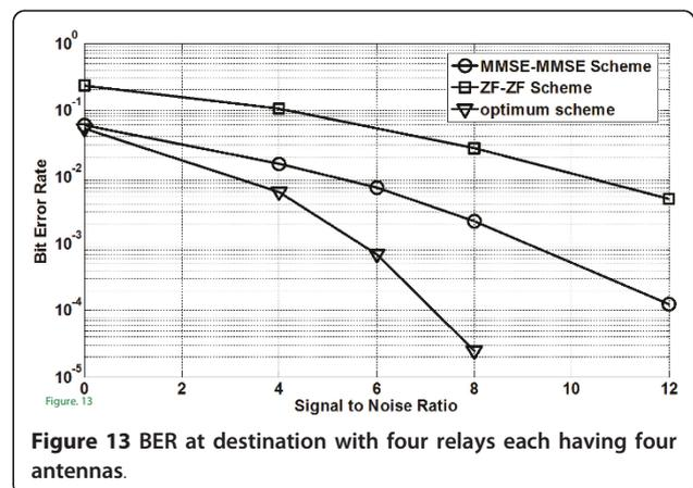
**Figure 13** BER at destination with four relays each having four antennas.
