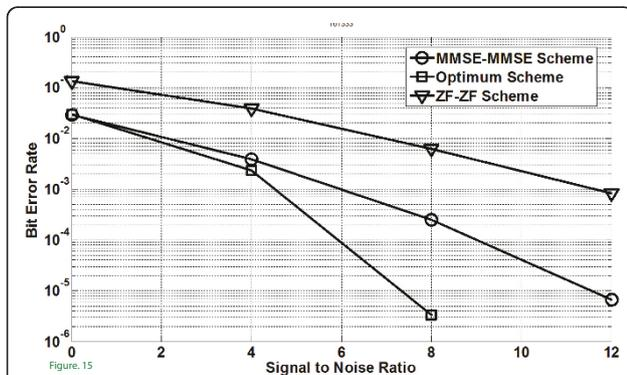
**Figure 15** BER at destination with six relays each having three antennas.
