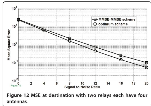
**Figure 12** MSE at destination with two relays each have four antennas.
