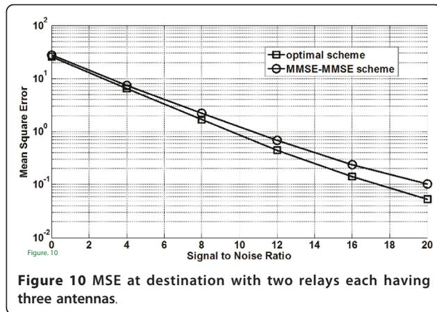
**Figure 10** MSE at destination with two relays each having three antennas.
