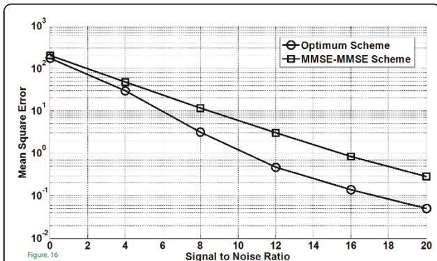
**Figure 16** MSE at destination with six relays each having three antennas.
