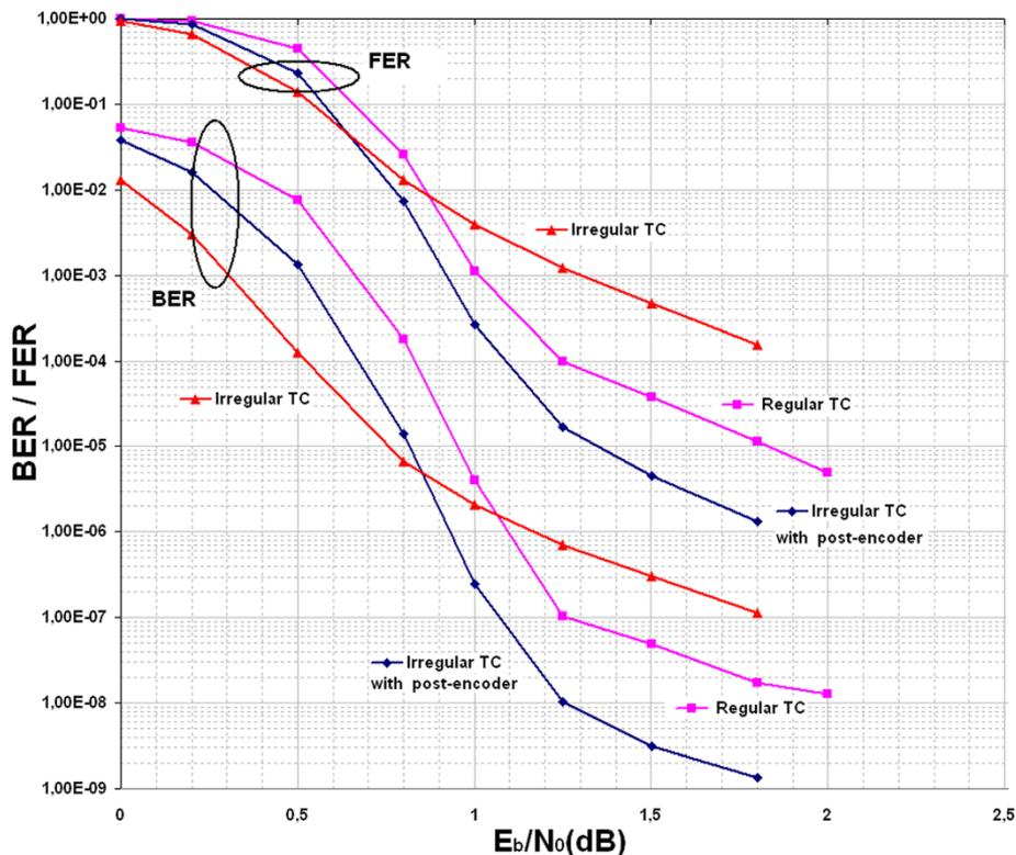
**Figure 8** BER and FER performance of 3GPP2 irregular TCs and comparison with the corresponding regular TCs. For blocks of 2,046 bits at coding rate  $R = \frac{1}{3}$ . The degree profile is  $(f_2, f_8)$ . All simulations use the MAP algorithm with 10 decoding iterations (transmission in a Gaussian channel).
