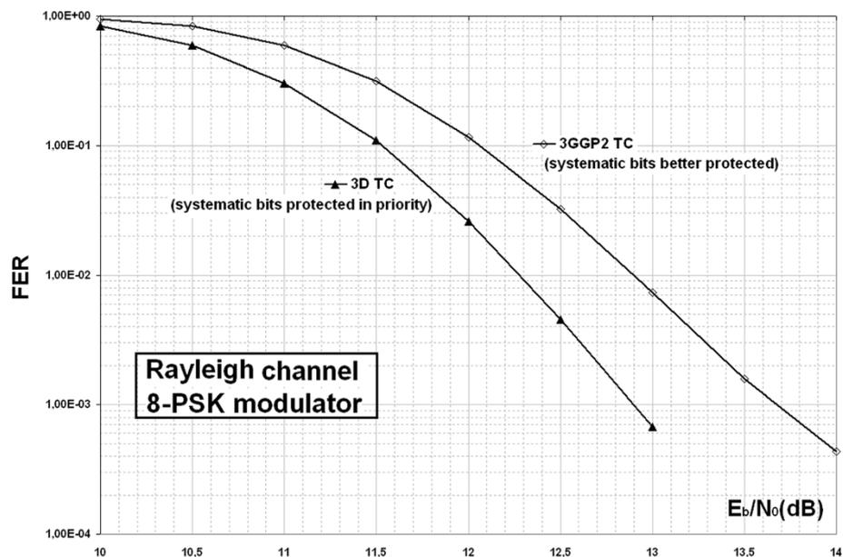
**Figure 4 3D TC associated with an 8-PSK modulator.** FER performance of the 3GPP2 3D TC with  $\lambda = \frac{1}{8}$  for  $k = 1,146$  bits,  $R = \frac{4}{5}$  and comparison with the 3GPP2 TC. All simulations use the MAP algorithm with 10 decoding iterations and 8-PSK modulation (transmission in a Rayleigh fading channel).
