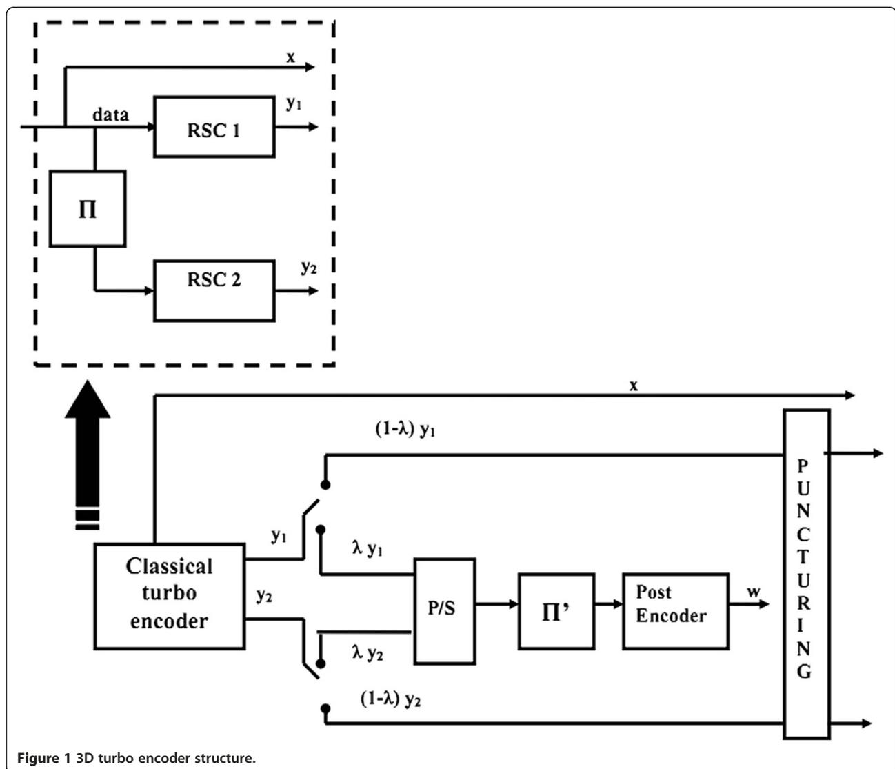
**Figure 1** 3D turbo encoder structure.
