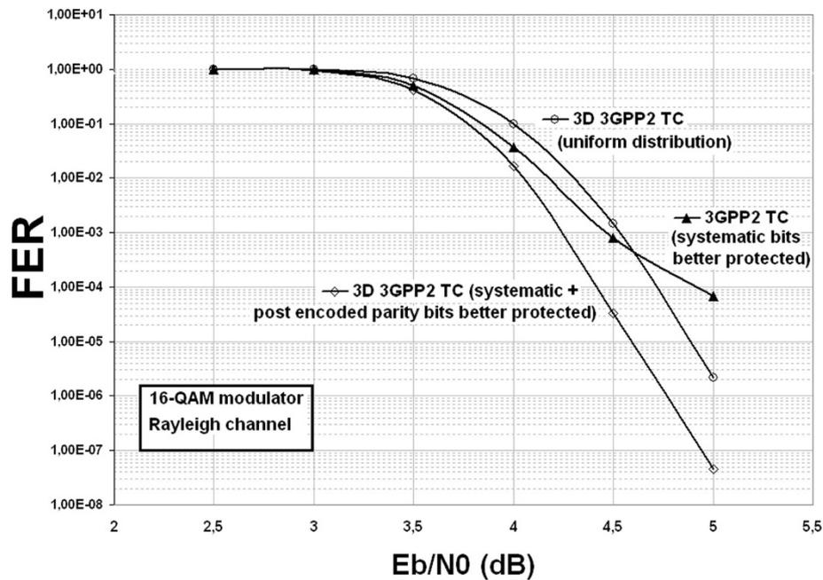
**Figure 3 3D TC associated with a 16-QAM modulator.** FER performance of the 3GPP2 3D TC with  $\lambda = \frac{1}{8}$  for  $k = 2,298$  bits,  $R = \frac{1}{3}$  and comparison with the 3GPP2 TC. All simulations use the MAP algorithm with 10 decoding iterations and 16-QAM modulation (transmission in a Rayleigh fading channel).
