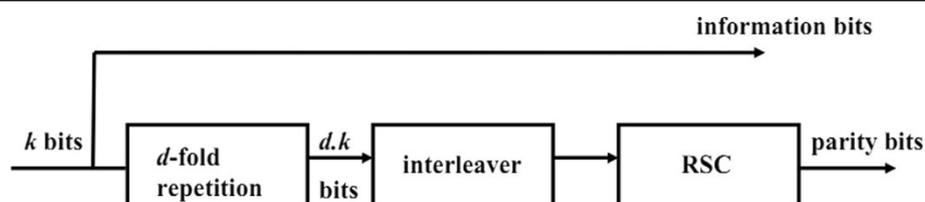
Figure 5 Equivalent encoding structure for a regular turbo encoder.
