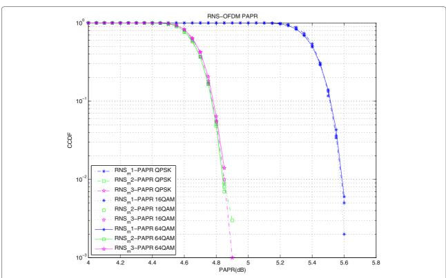
Figure 6 PAPR performance of the RNS-OFDM with 64QAM, 16QAM, and QPSK modulations.
