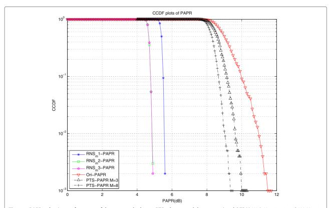
Figure 5 PAPR reduction performance of the proposed scheme, PTS scheme, and the conventional OFDM. With N=2,048,64QAM,  $V=3,W=\{-1,1\}$ , and M=3/M=8.
