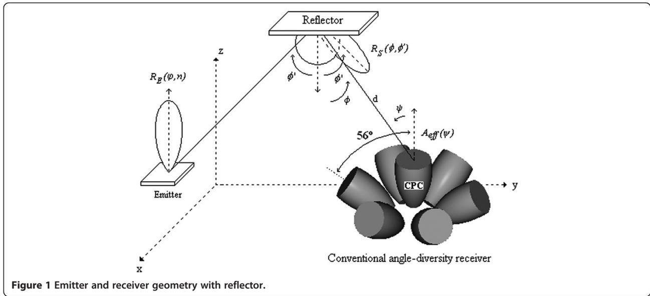
**Figure 1** Emitter and receiver geometry with reflector.
