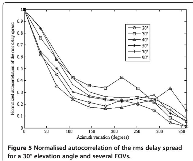
**Figure 5** Normalised autocorrelation of the rms delay spread for a  $30^\circ$  elevation angle and several FOVs.
