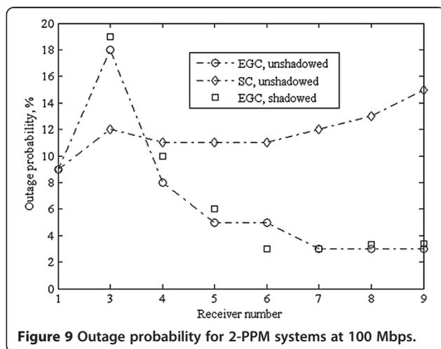
**Figure 9 Outage probability for 2-PPM systems at 100 Mbps.**
