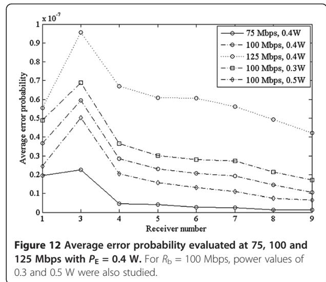
**Figure 12** Average error probability evaluated at 75, 100 and 125 Mbps with  $P_E = 0.4$  W. For  $R_b = 100$  Mbps, power values of 0.3 and 0.5 W were also studied.
