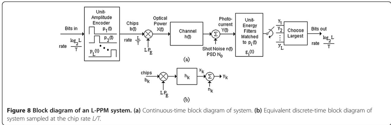
**Figure 8** Block diagram of an L-PPM system. (a) Continuous-time block diagram of system. (b) Equivalent discrete-time block diagram of system sampled at the chip rate  $L/T$ .
