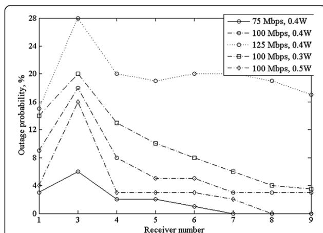
**Figure 11** Outage probability evaluated at 75, 100 and 125 Mbps with  $P_E = 0.4$  W. For  $R_b = 100$  Mbps, power values of 0.3 and 0.5 W were also studied.
