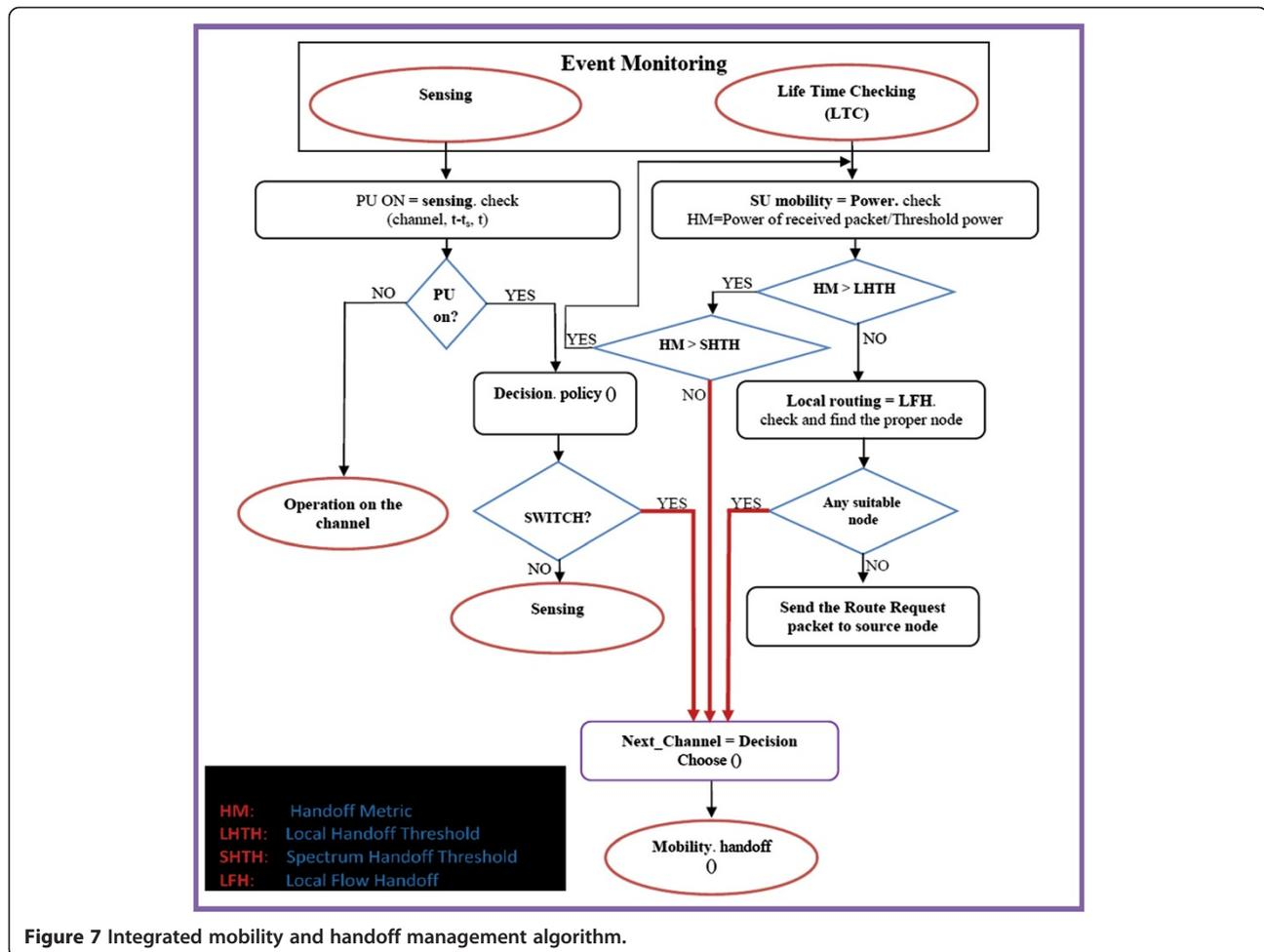
Figure 7 Integrated mobility and handoff management algorithm.
