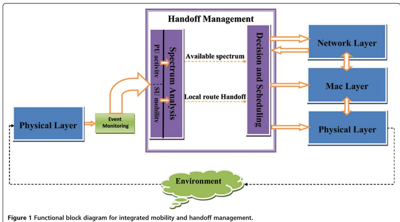
Figure 1 Functional block diagram for integrated mobility and handoff management.
