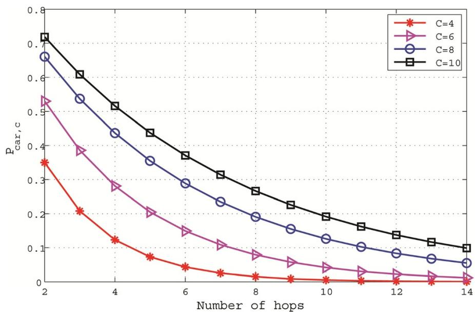
Figure 13 The effect of number of available channels on  $P_{car,c}$
