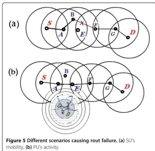
Figure 5 Different scenarios causing route failure. (a) SU's mobility, (b) PU's activity.
