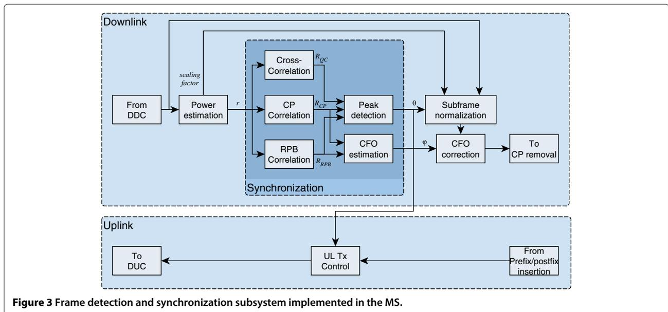
Figure 3 Frame detection and synchronization subsystem implemented in the MS.
