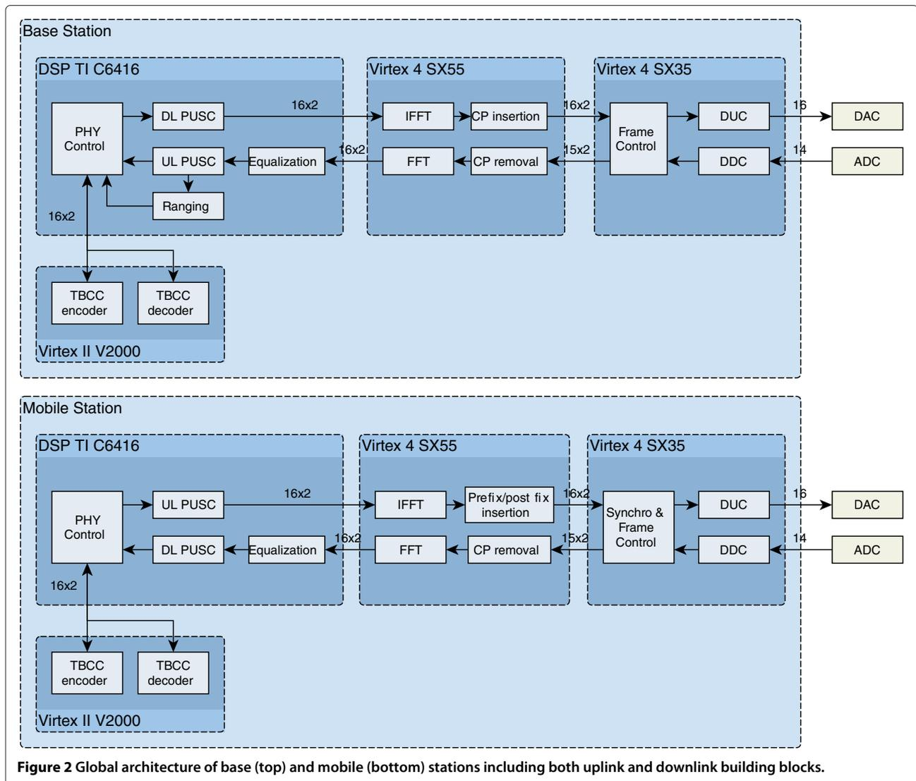
Two kinds of buses were used for communicating between modules: data buses and control buses. The latter are exclusively used for configuration messages. The throughput of the data and control buses is 400 and 20 MB/s, respectively. The communication between the host PCs and their corresponding carrier boards is done through the PCI bus.
