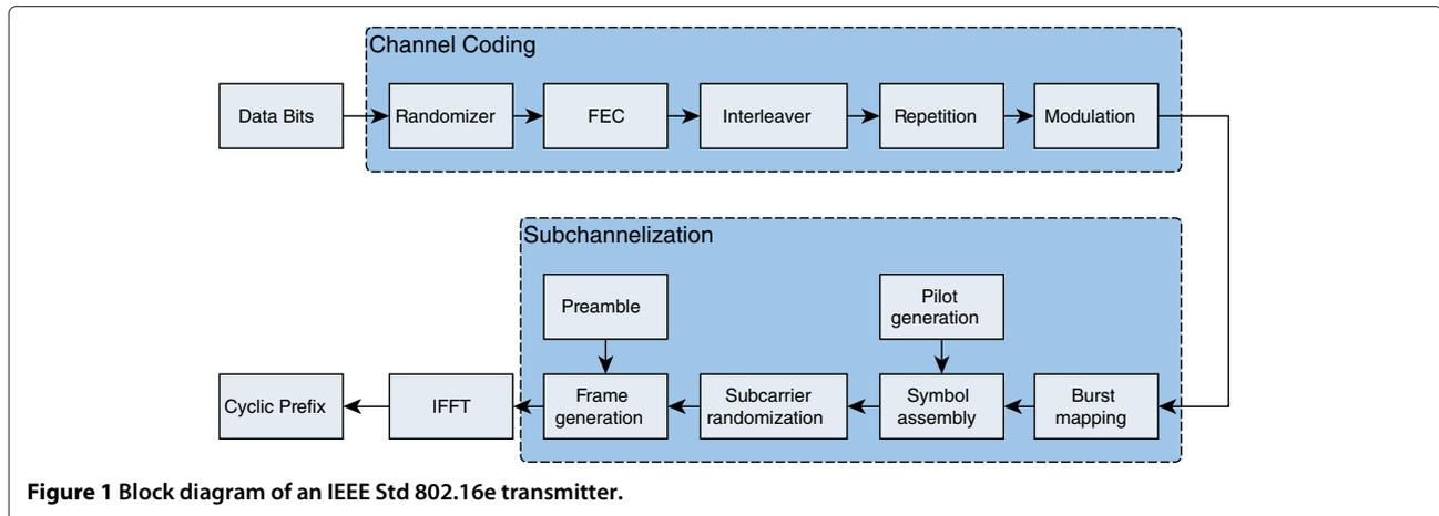
**Figure 1** Block diagram of an IEEE Std 802.16e transmitter.
