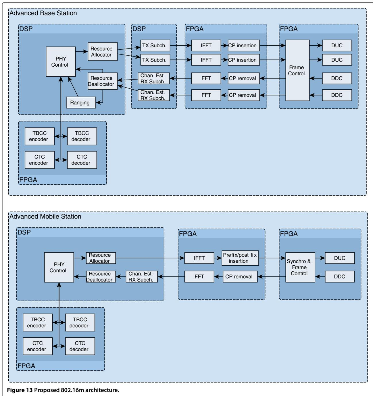
of downlink and uplink zones. Each subframe can be dynamically configured for downlink or uplink transmission. This dynamic behavior imposes the need to improve the *Frame control* block to be more flexible.
