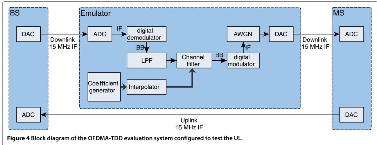
**Figure 4** Block diagram of the OFDMA-TDD evaluation system configured to test the UL.
