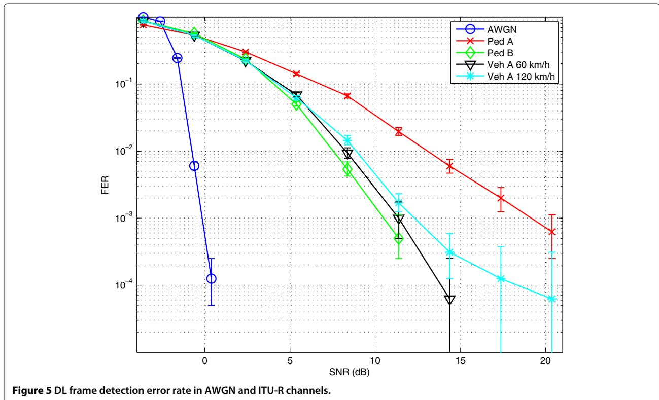
Figure 5 DL frame detection error rate in AWGN and ITU-R channels.
