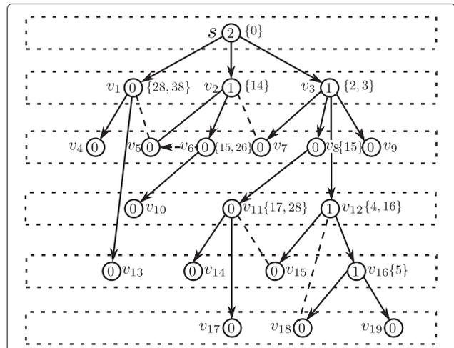
Figure 3 The ranking and broadcast scheduling of shortest path tree  $T_{\text{spt}}(G[U \cup C])$  consisting of solid edges. The number inside each circle is a node's rank, and the numbers in curly braces correspond to a node's transmission times.
