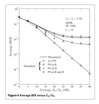
the PN at the destination introduces higher ICI to the useful signal, and consequently the worse performance is obtained. The OFDM system becomes more sensitive on PN in the high SNR region, and this difference is more evident. A fairly good agreement between the theoretical and simulated results is achieved, which confirms the validity of the performance analysis presented in this article.
