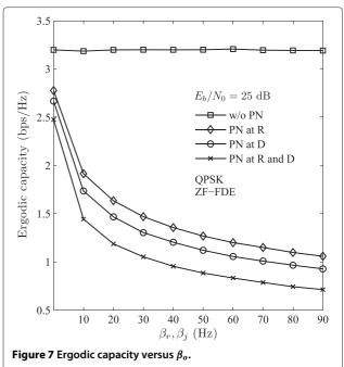
system's ergodic capacity. Moreover, the ergodic capacity is more sensitive to the PN encountered at the reception during the broadcast phase (i.e., at destination) in comparison to the reception during the multiple-access phase.
