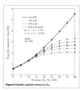
slope is particularly expressed for PN linewidth values in range (1-20) Hz. Furthermore, the difference between the obtained performance values is considerably constant (0.15 and 0.25 bps/Hz) for PN linewidth values in range (25-90) Hz.
