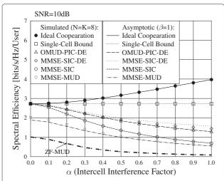
Figure 7 Spectral-efficiency versus intercell interference factor  $\alpha$  for the multicell systems with N=K=8 and operated at SNR = 10 dB.
