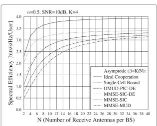
Figure 9 Asymptotic spectral-efficiency versus the number of receive antennas per BS for the multicell systems operated with  ${\sf SNR}=10$  dB and an intercell interference factor  $\alpha=0.5$ .
