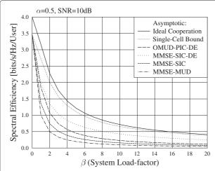
Figure 8 Asymptotic spectral-efficiency versus system load-factor  $\beta$  for the multicell systems operated with SNR = 10 dB and an intercell interference factor  $\alpha$  = 0.5.
