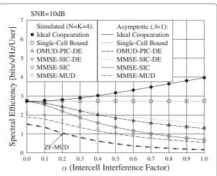
Figure 6 Spectral-efficiency versus intercell interference factor  $\alpha$  for the multicell systems with N=K=4 and operated at SNR = 10 dB.
