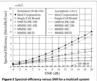
Figure 5 Spectral-efficiency versus SNR for a multicell system with the parameters N=K=16 and  $\alpha=0.5$ .
