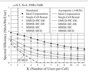
Figure 3 Spectral-efficiency versus the number of users per cell, when SNR = 10 dB, N=4 and an intercell interference factor  $\alpha=0.5$ .
