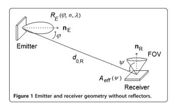
receiver, and FOV its field of view (semi-angle from the surface normal). In general, the emitter is modeled using a generalized Lambertian radiation pattern for each wavelength, and has axial symmetry (independent of  $\gamma$ )
