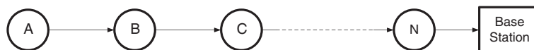
Figure 10 Multi-hop WSN. Node A transmits data to the base station through other nodes.
