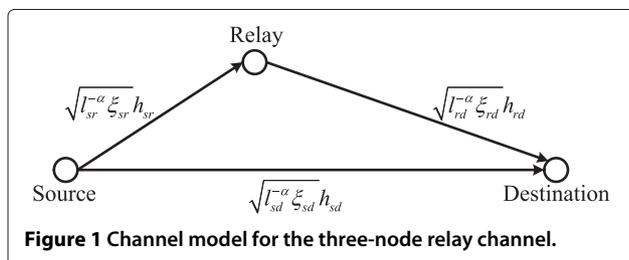
**Figure 1** Channel model for the three-node relay channel.
