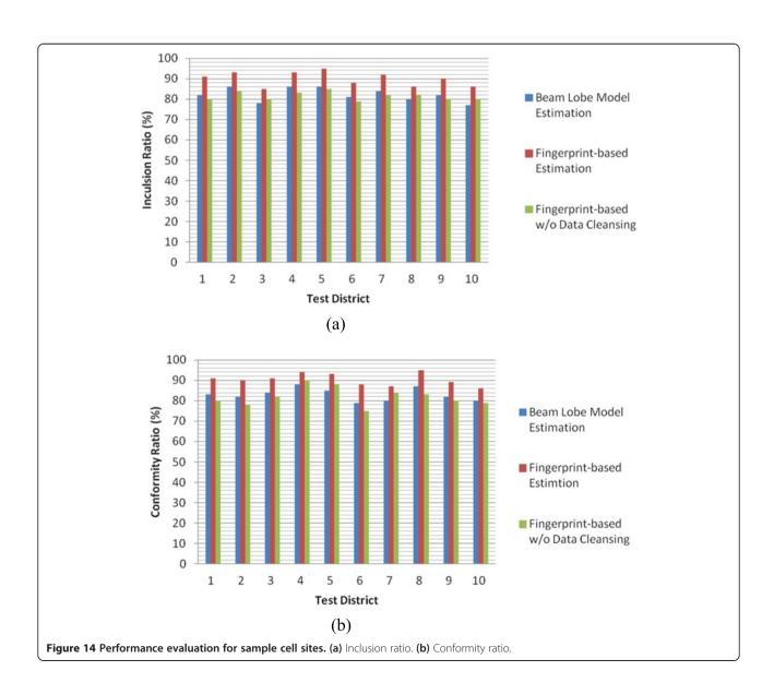
In addition, the proposed fingerprint-based estimation also improved the conformity ratio. The average value of the beam lobe model is 83.0%, and the fingerprint-based estimation is 90.4%, giving an improvement of 7.4%. Note that, we add the fingerprint-based estimation without data cleansing and compensation. There is no significant enhancement without data analytics: slightly lower performance is observed (-0.7% for inclusion ratio, -1.1% for conformity ration).
