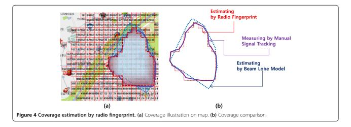
map and Figure 4b shows the difference between this method and other coverage estimation methods: beam lobe estimation and manual tracking.
