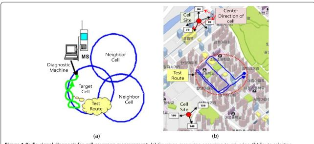
**Figure 1 Radio signal diagnosis for cell coverage measurement. (a)** Coverage measuring according to cell edge. **(b)** Route selection for measurement.
