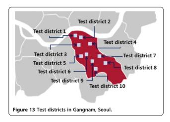
selected areas are collected by actual wardriving. Note that, the area of the Gangnam district is 39.55 km². The cell coverage estimation method was applied at 30 cell sites for each district. The total number of tested cells in Gangnam is 300, which is a sufficient sample size to show the effects of the proposed method in the entire area. For statistical analysis, a sample size of 300 to 400 cells is suitable. See the Appendix for details of the statistical conjecture.
